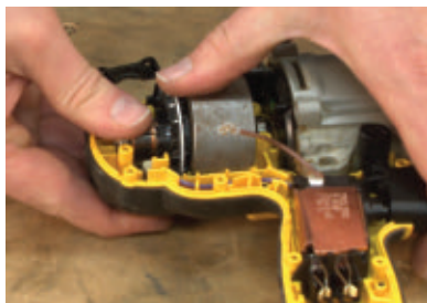
Replace motor and transmission assembly from drill
