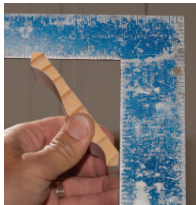
Read the scale on the framing square for the amount of wall and ceiling that is covered by the crown.
