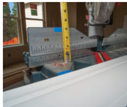
Use masking tape to mark the edges of the crown on the miter saw's table and fence so it is positioned at the correct angle to the saw blade.
