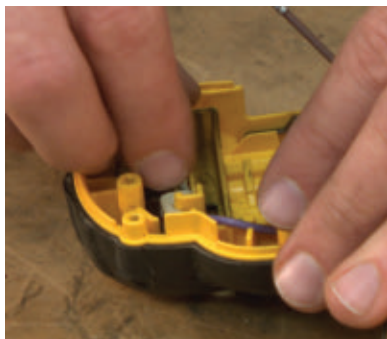
Replace brush and secure wiring
