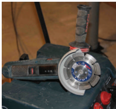
We used a grinder with a metal-cutting blade to cut the old columns.
