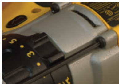
Replace remaining transmission screws
