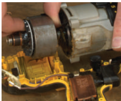
Pull motor and transmission assembly from drill
