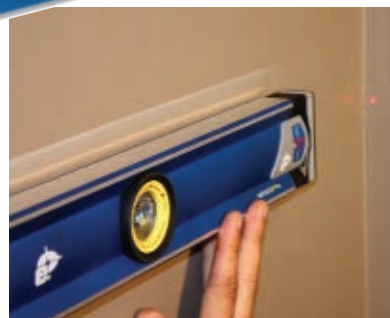
The e100 Series of box levels from Empire Level features a digital readout and a laser centerline that projects from the end of the tool.
