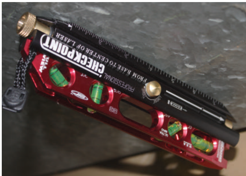
The CheckPoint Ultra-Mag G3 torpedo level with Ultra Mag Laser Base broadcasts a Class II pinpoint laser beam that is accurate up to a 1/4" over 100'.
