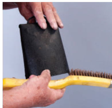
Clean off the treated item. As you can see in the lead photo, most of the oxide is soft and easily powders off the cow bell.
