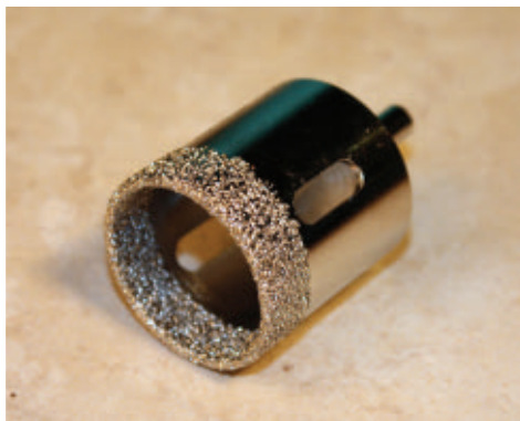
Diamond-tipped hole saws make circular cuts in tile for pipe and cable access.
