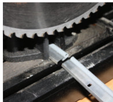
Cut the strip to length. I used a chop saw, but a hacksaw works best.
