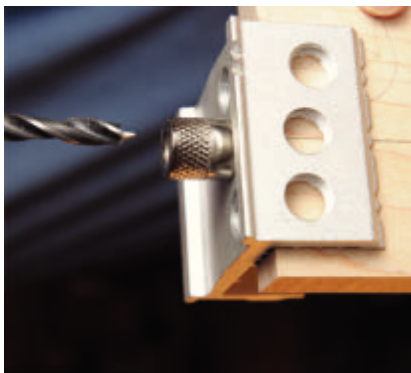
Alignment indicators on the jig ensure perfect alignment of dowels on board edges or ends, as shown here.
