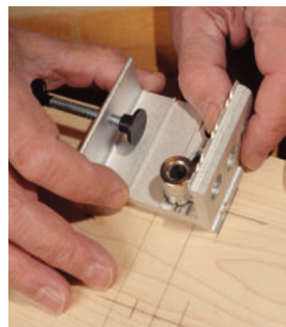
The E-Z Pro doweling jig can be quickly reconfigured and repositioned for placing dowels in any location, including board centers.
