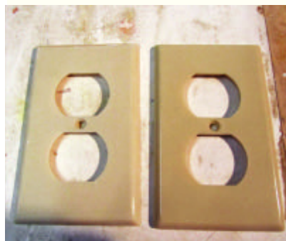
Sanding de-glosses and etches the surface so the primer adheres better.
