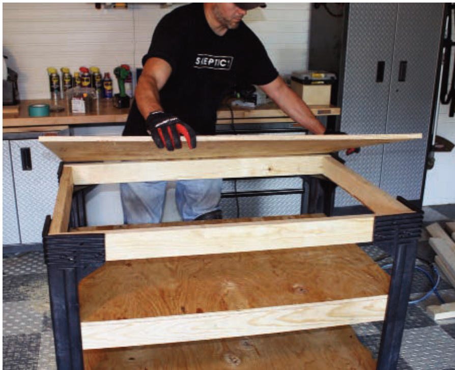
Last step is to screw on the 3/4" plywood table top.
