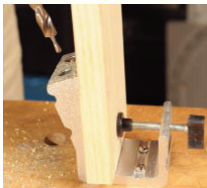
Pocket-hole joints are a snap to make with this jig. The stepped drill bit and adjustable stop collar are included with the jig.
