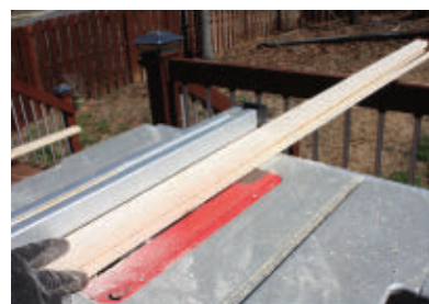
Make intersecting partial rips to cut the rabbets.
