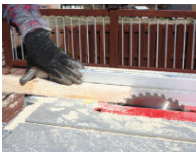
Rip 2x4's into 2x2's and square the edges of the 2x stock.
