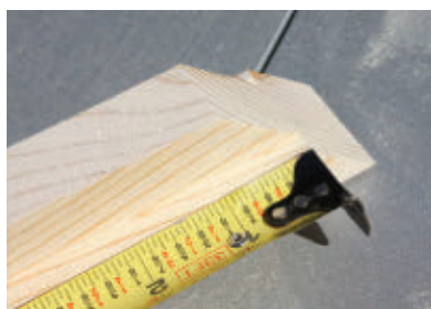
When measuring for the plywood, take the measurement from the corner of the rabbet, not the outside corner of the stock.
