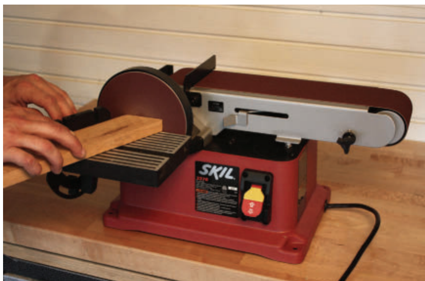
The Skil 3376 benchtop unit is a versatile combination of a stationary sanding disc and 4x36" belt. It's a handy tool for detail work such as sanding small end surfaces with the disc.
