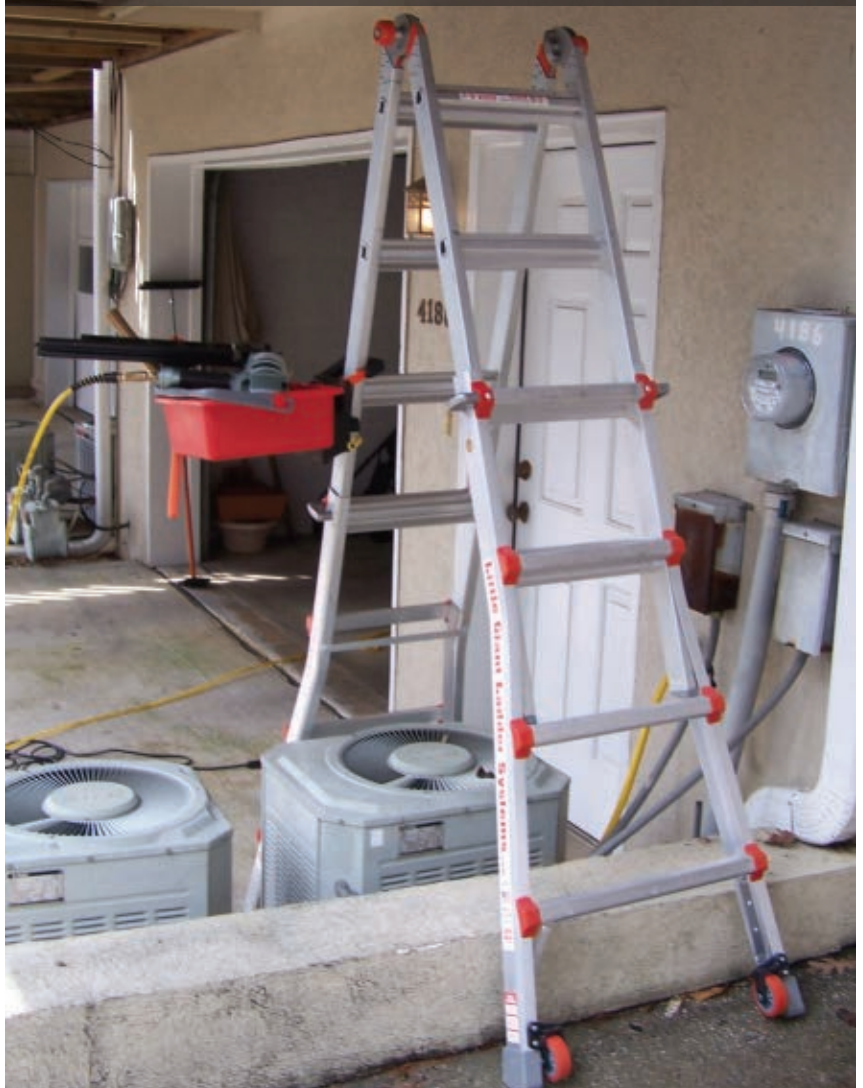
Each side of the Little Giant Ladder can be independently adjusted for length, so it can bridge uneven footing and obstructions like the curb and air-conditioning unit shown here.
