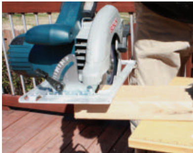
The saw base of the CS5 overhangs the work-piece when trimming the end, which takes a little practice.
