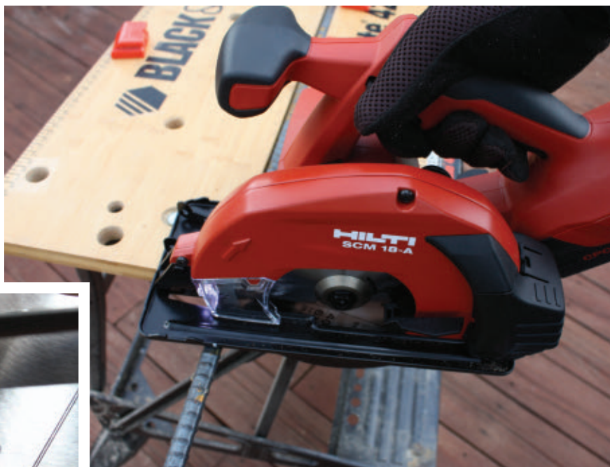
The Hilti SCM18-A is a cordless 18V metal-cutting saw that slices through 5/8" rebar with ease.
