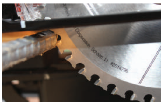
The Hilti SCM18-A is a cordless 18V metal-cutting saw that slices through 5/8" rebar with ease.
