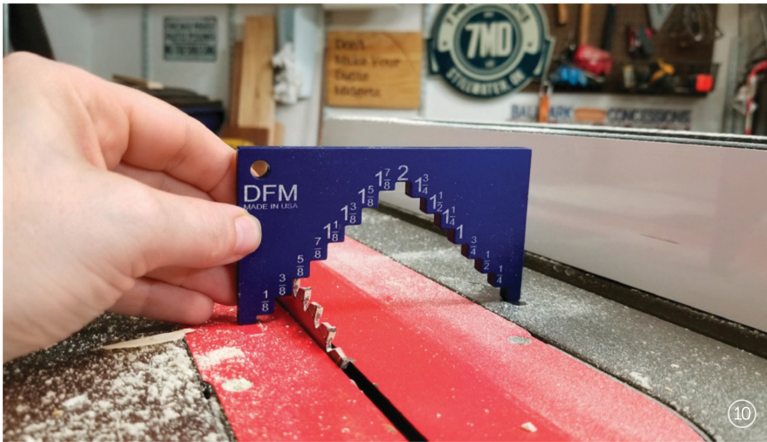
10. SAW HEIGHT GAUGE The aluminum laser cut and anodized tool helps set the height of a table saw within \frac{1}{64} -inch accuracy. $20; dfmtoolworks.com
