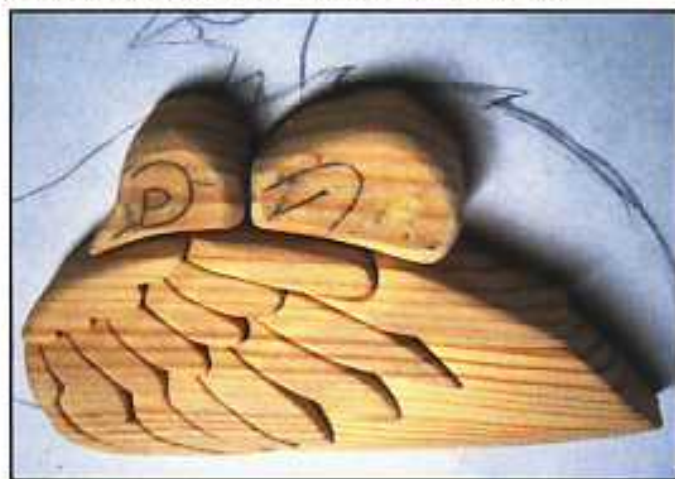
Step 13. The resting chick section needs to be slightly thinner than the mother's wing. Use the belt sander to carefully sand down the piece from the back side. Cut apart the head and body, and then shape and sand the two pieces.
