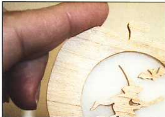
Step 20. When correctly positioned, the edges of the plexiglass should not be visible when the assembly is viewed from the front. Allow the glue to dry completely.
