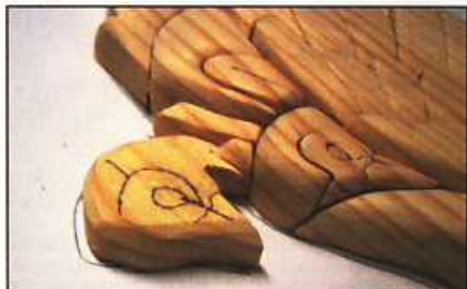
Step 17. Use the belt sander to carefully sand down the back side of the second chick so that the piece is slightly
