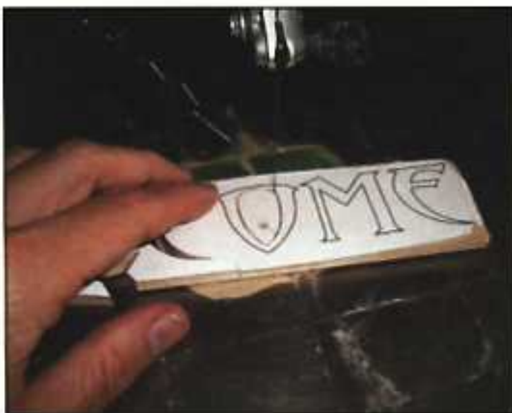
Step 8. Use the No. 2/0 reverse-tooth blade to cut out the letters.
