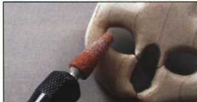
Step 12. A conical-shaped tip for rotary sanding tools is useful for shaping hard-to-reach areas such as the inner sections of the eye and nose areas. Alternatively, those areas could be hand-sanded.
