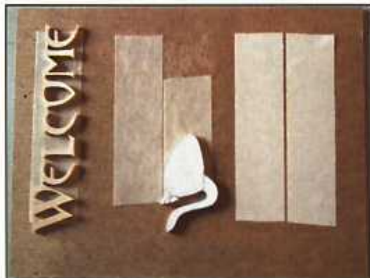
Step 9. As you cut the letters and overlay pieces, it is helpful to attach them to strips of double-sided carpet tape that has been adhered to some scrap wood. This keeps all the pieces organized and aids in the assembly process.
