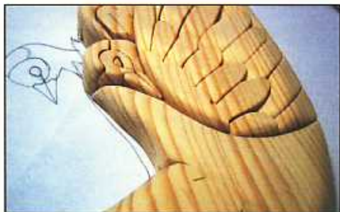
Step 15. Use the belt sander to taper the edges of the mother's chest piece. The edges of the chest piece should be thinner than the adjacent neck and wing pieces. Also taper the edge of the chest section where it contacts with the resting chick's head, in order that the baby sits a bit above the chest. Gradually round the edges of the chest so that it is nice and smooth.
