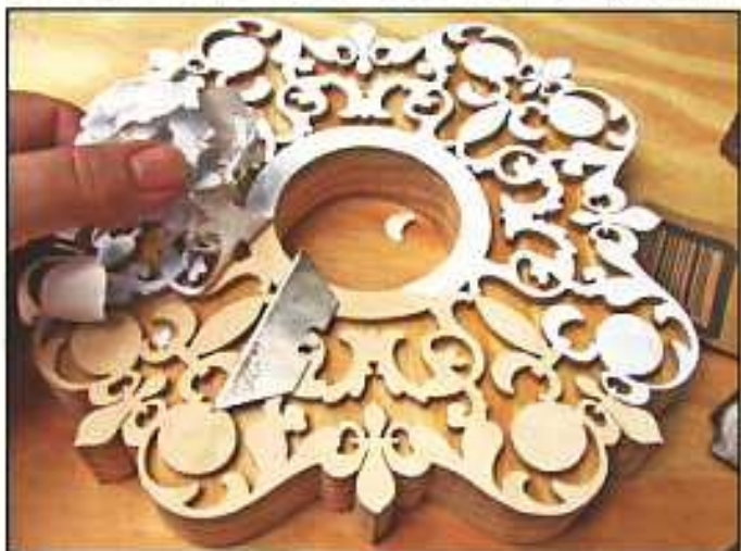
Step 13. Remove the patterns and tape. Carefully separate the backing and overlay pieces. Hand-sand the pieces, starting with 150-grit sandpaper, and progressing through 220-grit and 320-grit until the surfaces are smooth. Remove all sanding dust using a hard-bristled paintbrush.
