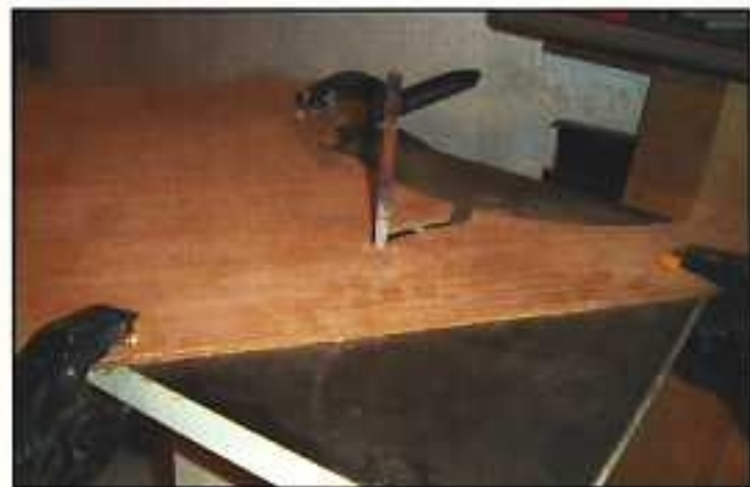
Step 5. First, I clamp a piece of plywood over the sander to eliminate any clearance to the drum.
