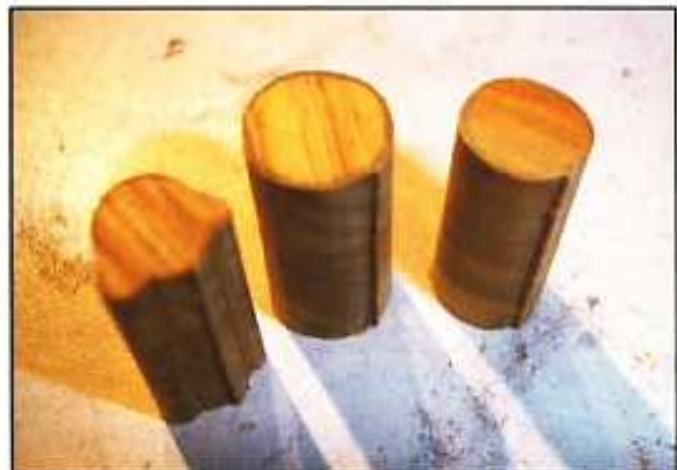
Step 4. For this next step, the spindle sander becomes my new best friend! Note the entry and entrance marks left by the saw on the cut pieces—the spindle sander is great for removing them. Also, it is imperative that the cuts are square to the bottom of the piece, otherwise the sections won't fit together properly. It is possible that the cuts are not perfectly vertical, either due to poor cutting technique, dull blades, or just very tough wood. The spindle sander comes in handy for squaring up those cuts.
