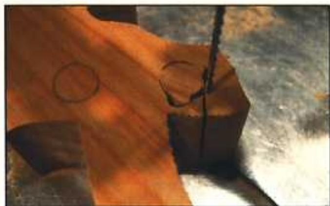
Step 3. Cut out the three pieces using the scroll saw.
