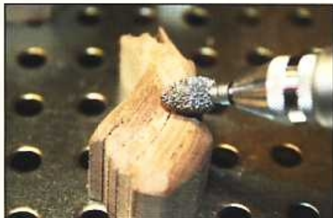
Step 16. Use a rotary tool fitted with a coarse shaping burr to give the grass pieces a rougher texture.
