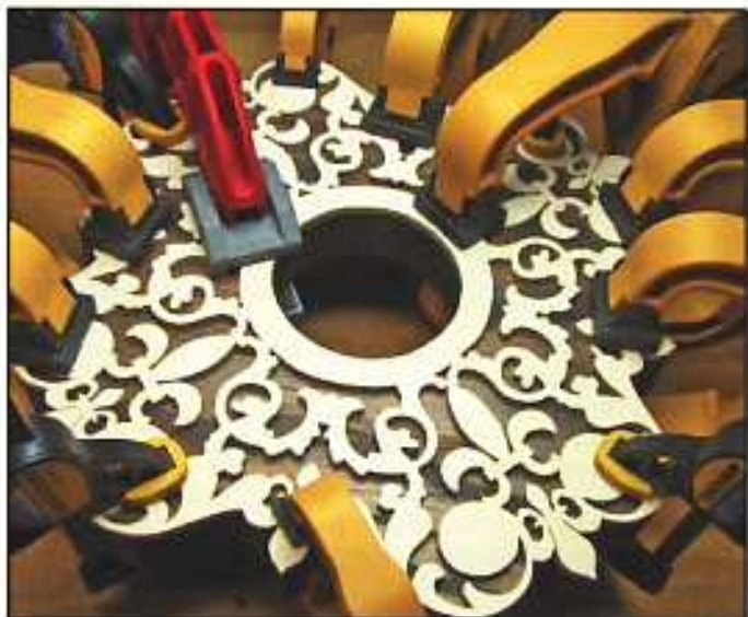
Step 16. Position the overlay on top of the backing. Apply clamps, and allow the assembly to dry.
