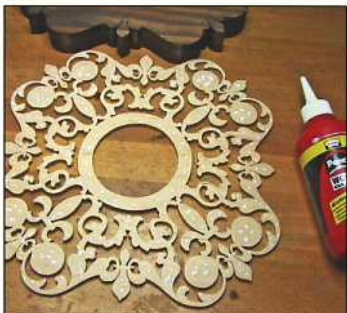
Step 15. Apply small beads of wood glue to the back of the overlay piece.
