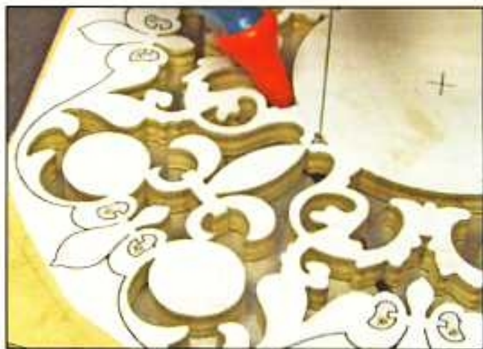
Use smallest-size blade possible to cut delicate areas.
