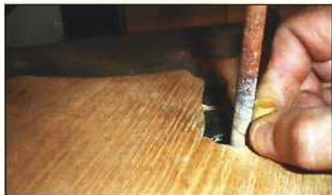
Step 6. Using the 1/4" spindle, I repair the entrance/exit saw marks and I sand all the edges around the piece, ensuring they are square.
