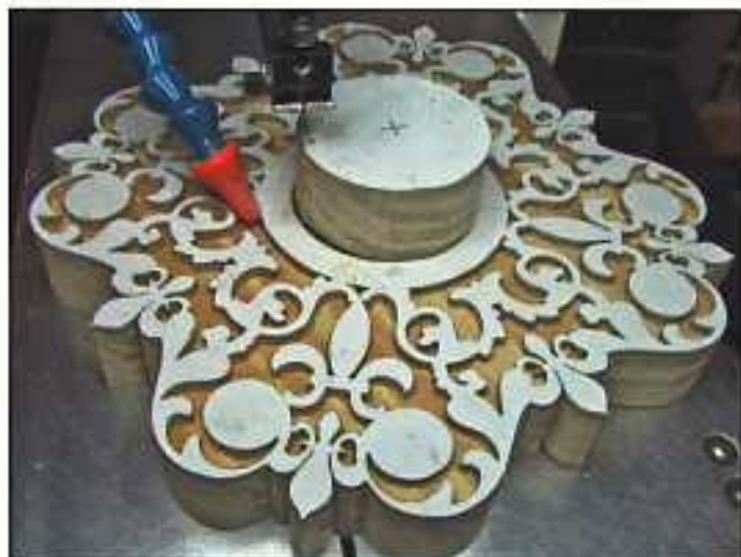
Step 12. Using the 3/32" bit, drill the blade entry hole for the clock opening. Cut out the opening, and test fit the insert. Cut or sand the opening as needed to achieve a proper fit.
