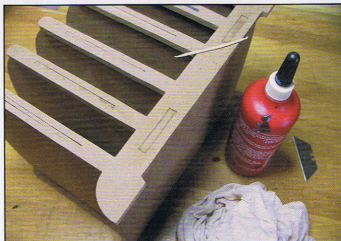
Step 21. When all six dividers are in place, turn the assembly on its side, and glue the other side panel in place. Remove any excess glue using a damp cloth. Allow the stand to dry.
