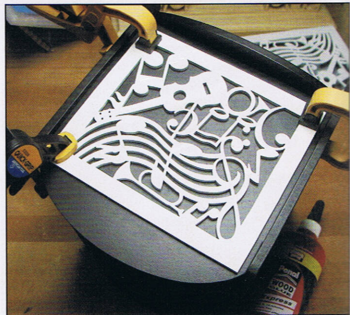
Step 24. Use wood glue to secure the stand overlay to the front of the stand. Apply clamps, and allow the glue to dry completely.
