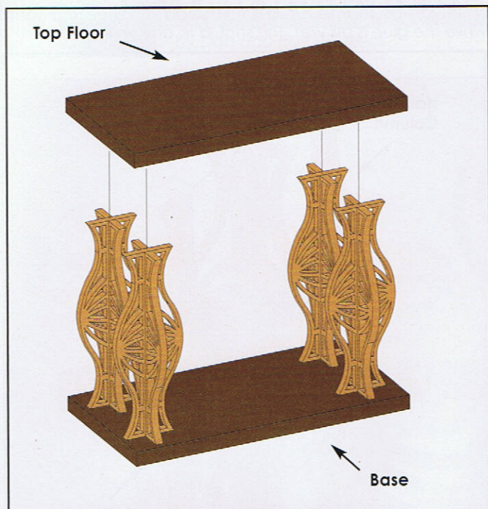
Step 7. Center the Top Floor on the column assemblies, and glue in place.
