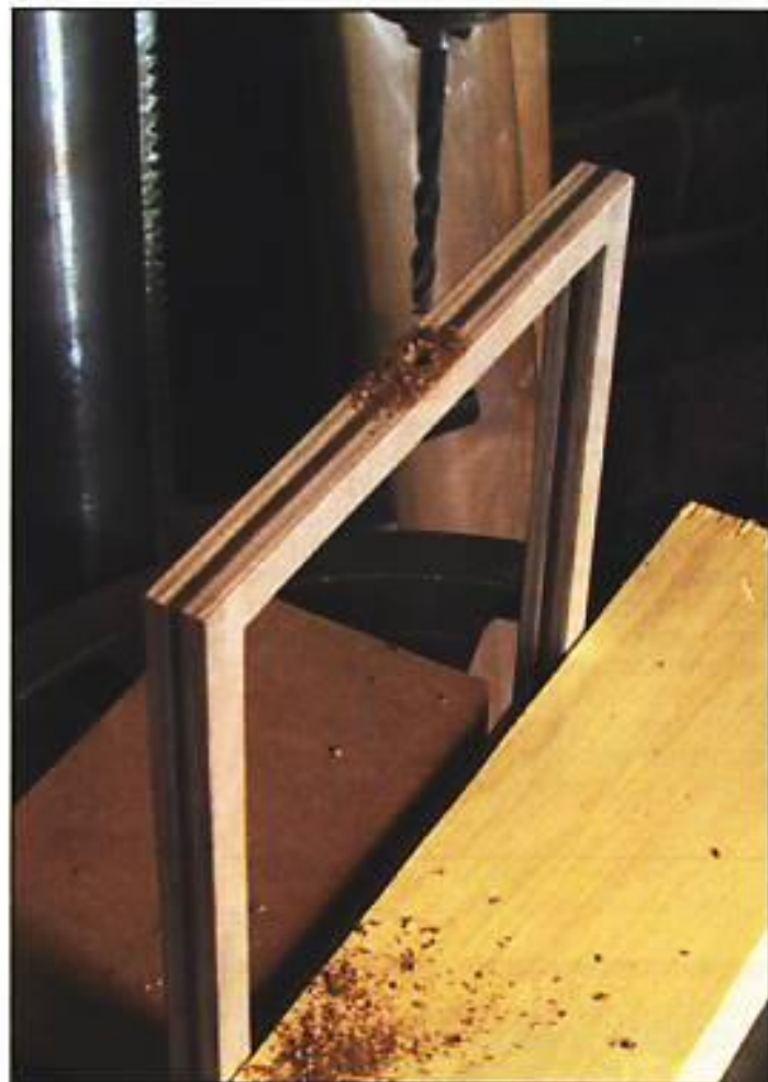
Step 23. Locate the center points along the top and bottom edges of the outer frame, and mark the points using a punch tool. Drill holes at both points using the 3/16" bit.
