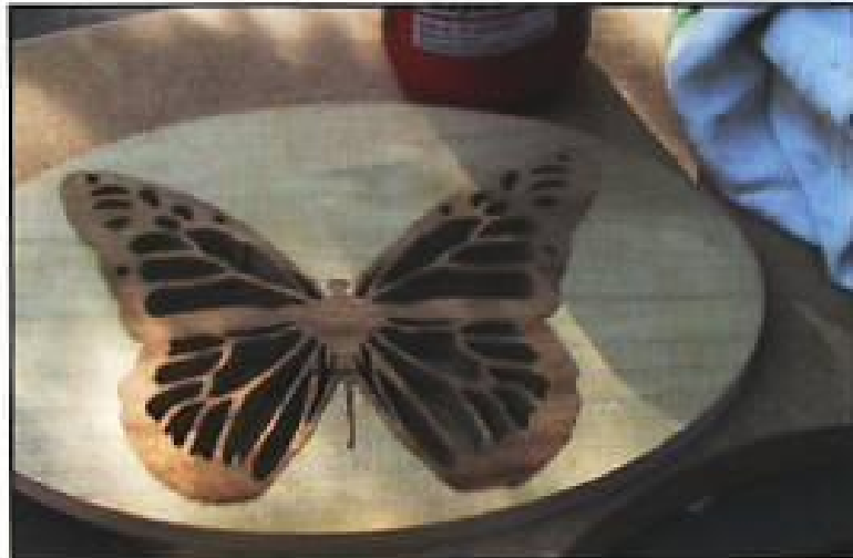
Step 13. Use wood glue to secure the inlay piece in the box lid opening. Remove any glue seepage using a damp cloth.
