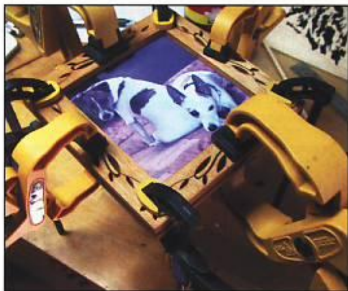
Step 22. Apply beads of wood glue to the plywood inner frames, press them into place on each side of the MDF interior layer, and clamp until dry.
