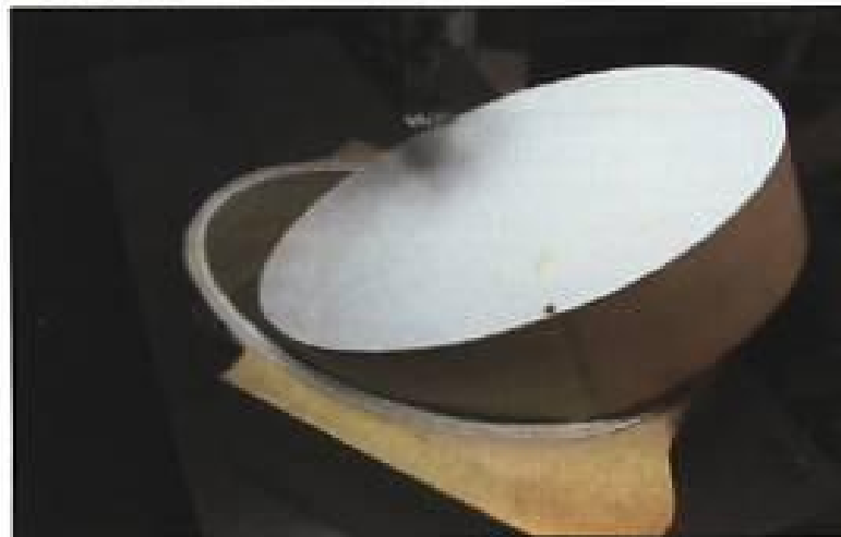
Step 9. Thread the No. 12 blade through the blade entry hole, and cut the interior opening for the box sides.
