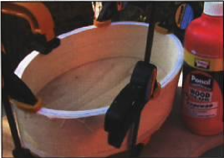
Step 11. Position the box sides piece on the box bottom, and glue in place. Attach clamps to secure.
