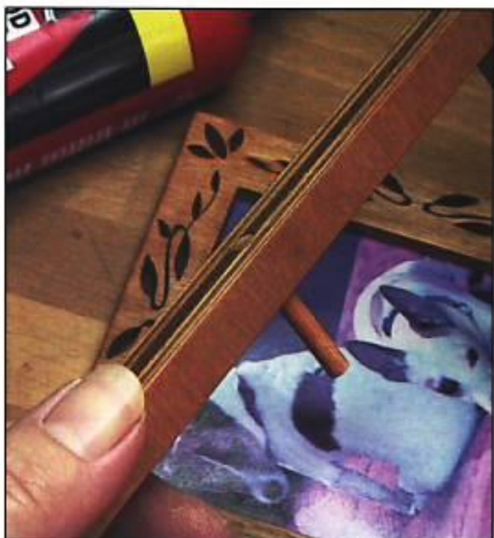
Step 25. Cut a 1-3/8"-long piece of dowel, and insert it into the top opening on the outer frame until the dowel is flush with the top edge. Glue it in place using wood glue.
