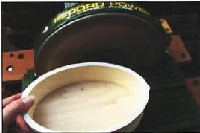
Step 12. Using the disc sander, sand the edges of the box assembly and lid up to the pattern lines. Remove all tape and patterns.
