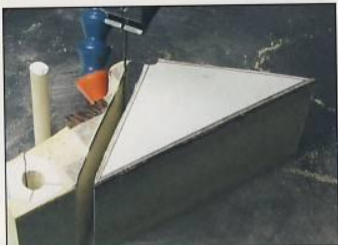
Step 12. Using the No. 12 reverse-tooth blade, cut out the roof work piece 1/8 " beyond the pattern line.
