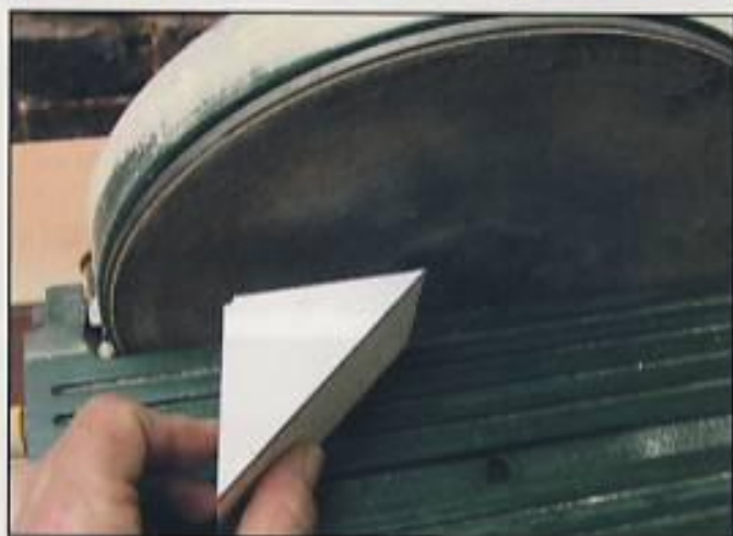
Step 18. Using the disc sander, sand up to the pattern lines on the clock body and roof pieces.
