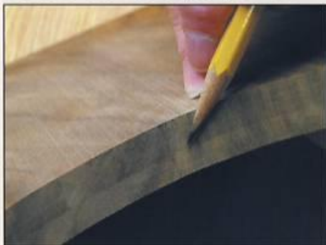
A visible line may be left on the edge of solid woods when sawing with reverse-tooth blades.
