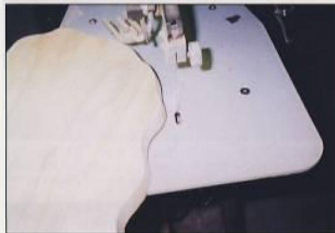
Step 17. Trace the base pattern onto the wood. Cut along the traced line at a 30° angle so the sides slope out. Set the base aside.
