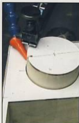
Step 15. Drill the blade entry hole using the 1/8" drill bit, and cut out the circular opening.
