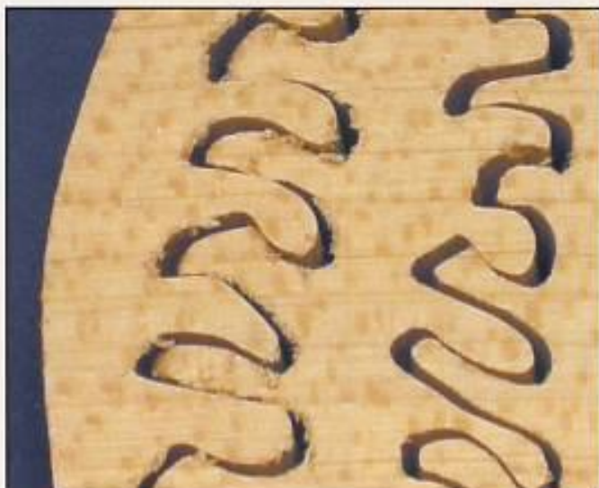
Skip-tooth blade cut line on left, reverse-tooth blade cut line on right
