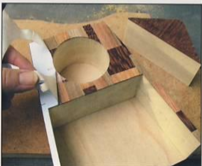
Step 19. Remove the patterns from the clock body and roof pieces by peeling off the masking tape.
