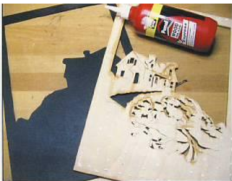
Step 16. Use wood glue to assemble the layers of the project. First, glue the middle layer to the painted middle layer backing piece, being sure to align all outer edges.
