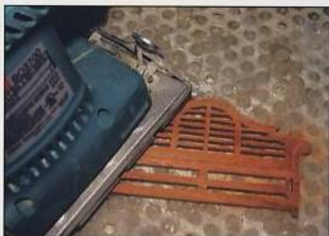
Step 7. Using the handheld orbital sander and fine-grit sandpaper, carefully sand the backs of the overlays.
