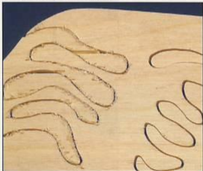
Skip-tooth blade cut line on left, reverse-tooth blade cut line on right
