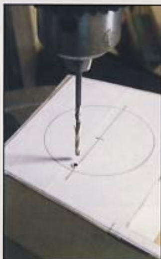
Step 15. Drill the blade entry hole using the 1/8" drill bit, and cut out the circular opening.
