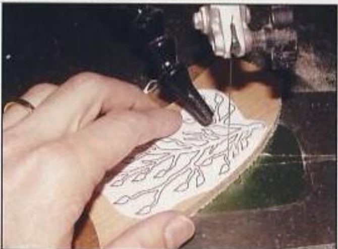
Step 6. Using the No. 2 reverse-tooth blade, cut out the overlay pieces. Cut the inner veining lines first, and then cut the perimeter of the pieces. The pieces will be very delicate, so handle them with care.
