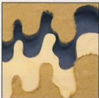
Thin cardboard can be used as a backer board to keep the bottom side of a project clean.
