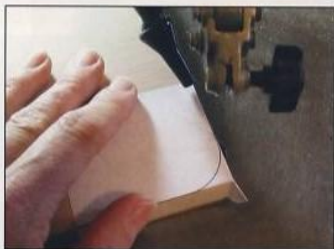
Step 8. Ensure that all edges of the backboard are cut to square. Position the rounded corner guide pattern on each corner, and cut along the line using the scroll saw. When finished cutting, sand the edges to remove any entry or exit marks made from the scroll saw blade.
