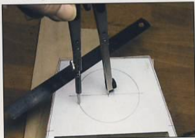
Step 14. Measure the opening required for your clock insert, and use a compass to draw the correct-sized opening in the center of the clock body piece.
