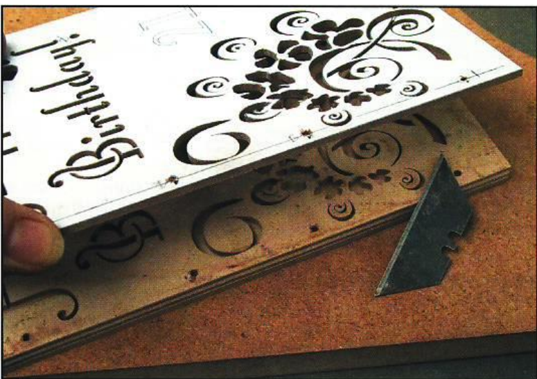
Step 9. Pry apart the work pieces by inserting a scraper blade between the layers.
