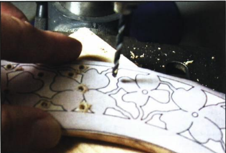
Step 11. Using a small drill bit, drill all the entry holes of the apple blossom design. (I matched the bit size to the size of the center of the apple blossoms.)
