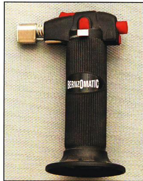
Step 6. After sawing, remove the pattern and all the tape. Blow off the sawdust. Use a mini-torch to burn off the "fuzzies" from the back-side. Caution: Keep the torch moving to prevent charring the backside, and DO NOT use the torch if you have applied any type of solvent or finish to your wood up to this point.
