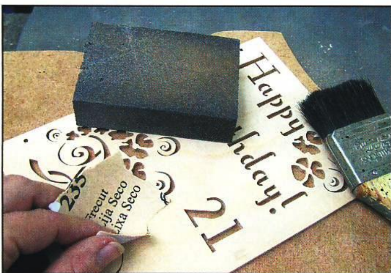
Step 10. Drill the holes for the numbers on the individual card fronts, and make the cuts. Remove the masking tape and patterns. Use a medium-grit sanding sponge to remove any burrs from the work pieces. Sand the pieces using 150-grit sandpaper and graduate to 320-grit, until you have achieved a smooth finish. Be careful not to
