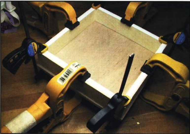
Step 8. Place the box frame on top of the base piece, and clamp to secure. Use a scraper blade or other method of choice to remove any glue seepage from the interior of the box. When dry, remove the clamps.
