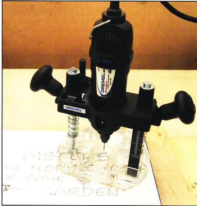
Step 3. Drill all the necessary blade entry holes in the waste areas. (The Dremel works nicely for this task, but be aware that the drill bit collet is a separate accessory.)
