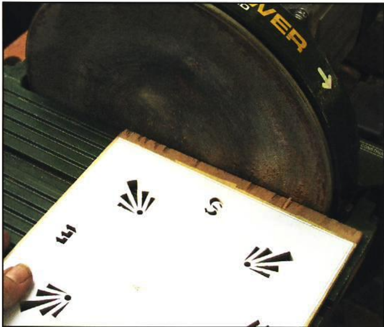
Step 11. Use the disc sander to sand up to the outer pattern line of the box lid.
