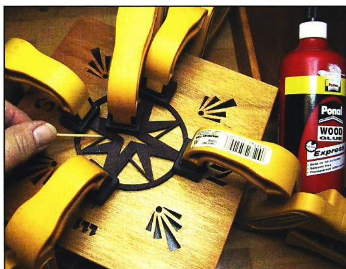
Step 18. Apply wood glue to the back of the overlay. Center it on the front of the lid, and clamp to secure. Use a toothpick to remove any glue seepage.
