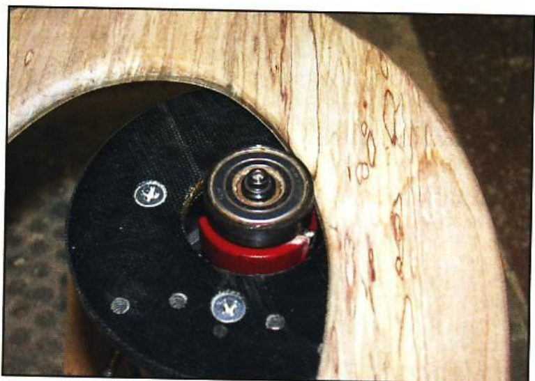
Step 9. Install the 1/8" rabbet bit in the router, set the depth to 1/8", and rout the inner back edge of the frame.
