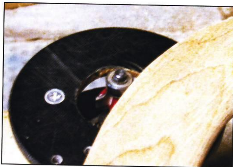
Step 8. Rout the outer front edge of the frame using the same bit and depth.
