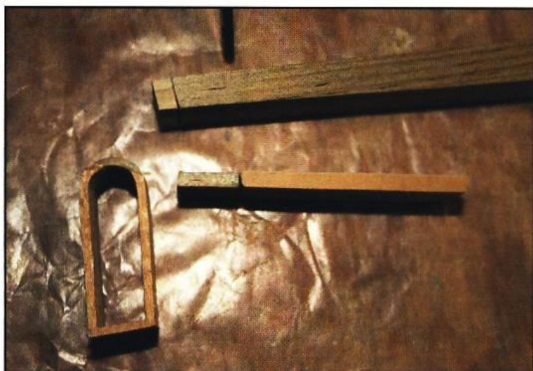
Step 9. Glue the shadowed pieces together, then carefully remove the patterns and shape each side down 1/16" toward each corner to add depth. Reattach the patterns, and cut apart the separate boards of the church siding at this point.
