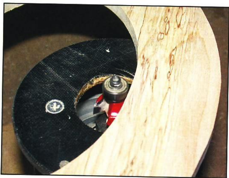
Step 7. With a slight roundover bit in the router, rout the inner front edge of the frame. (You will know the front from the back because the penciled reference mark was placed on the back of the frame in the previous step.)
