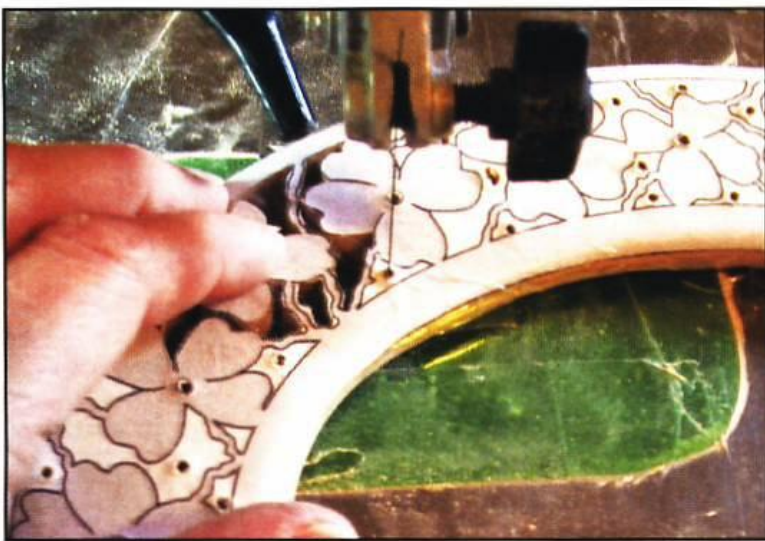
Step 13. Use the No. 2 reverse blade to cut out the design. When finished, gently sand the frame using fine-grit sandpaper.
