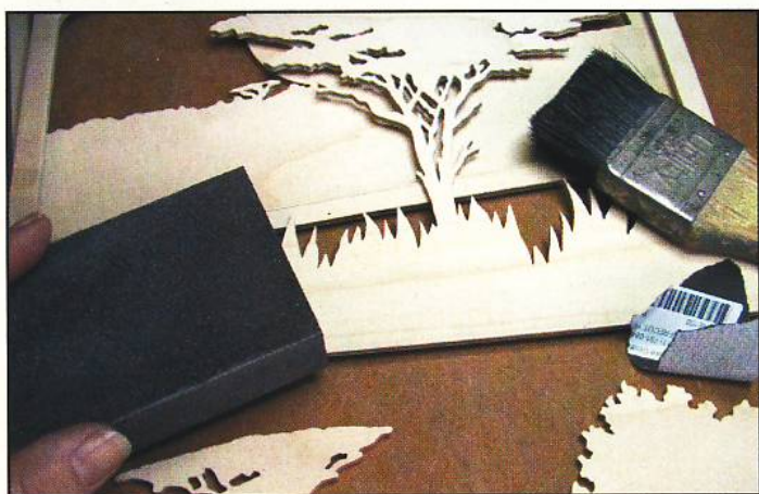
Step 8. Use a medium-grit sanding sponge to remove any burrs from the work pieces. Sand the pieces, first using 150-grit sandpaper, then 320-grit, until you have achieved a smooth finish. Be careful not to catch and break any fragile pieces. Use a hard-bristled paintbrush and a lint-free cloth to remove all sanding dust.
