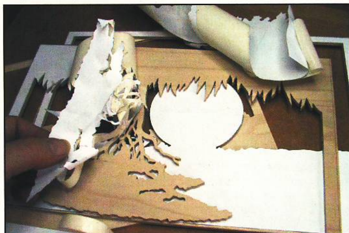
Step 7. Remove the patterns by peeling off the masking tape.
