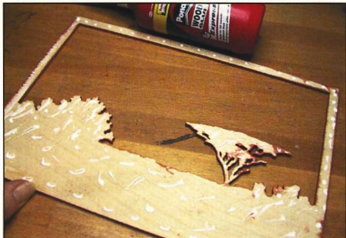
Step 13. Apply small beads of wood glue to the back of the middle layer, and position it on top of the bottom layer.
