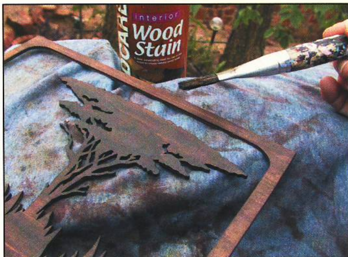
Step 10. Apply walnut wood stain to the front and edges of the top layer. Use a medium-size artist's brush to apply the stain in order to reach all the inner surfaces of the pierce cuts.
