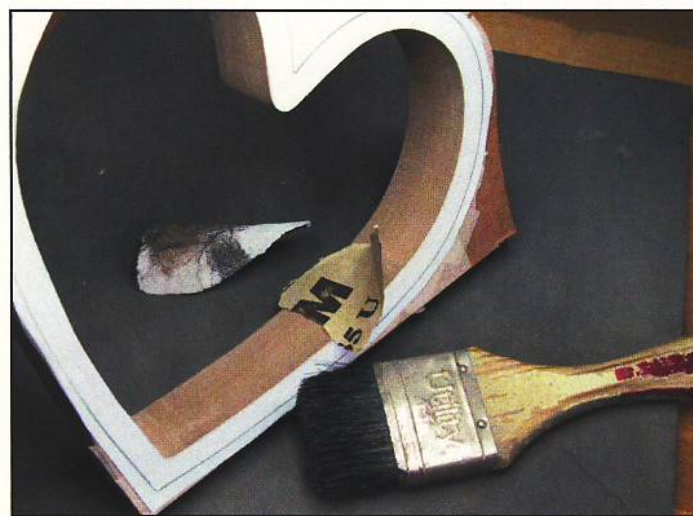
Step 9. Using first 150-grit, and progressing through 320- and 500-grit sandpaper, hand sand the interior surfaces of the box body until you achieve a smooth finish. Remove all sanding dust.
