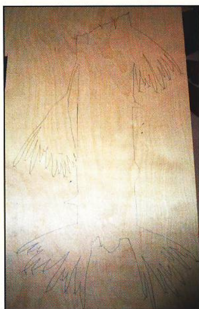
Step 17. After completing the tracing, attach the pattern to the plywood. Drill all pilot holes. Cutting 1/16" to the inside of the traced lines, cut out the backer.
