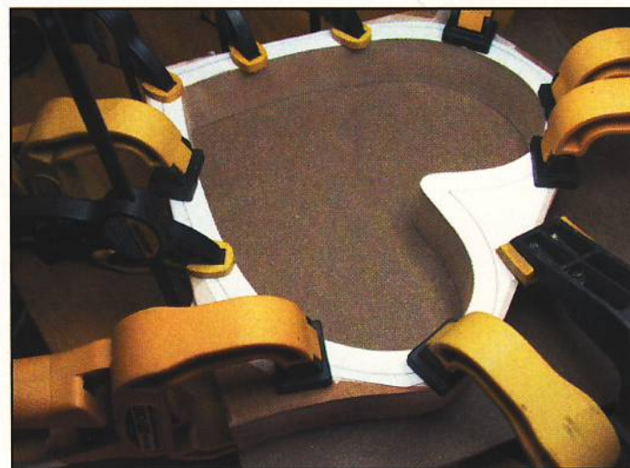
Step 11. Place the box body on the base work piece, and clamp together. Use a toothpick, scraper blade, or damp cloth to remove any glue seepage from the inside of the box. When dry, remove the clamps.
