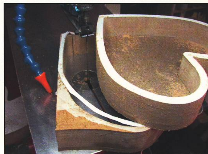
Step 12. Using the scroll saw and the No. 12 reverse-tooth blade, cut along the outer line of the box body pattern, cutting through both the box body piece and the base.
