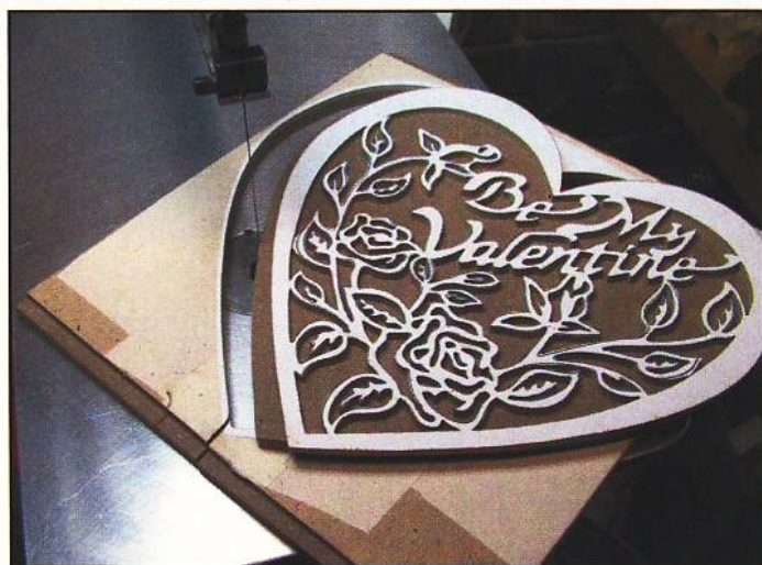
Step 8. Using the No. 3 reverse-tooth blade, cut the perimeter of the pattern. Separate the two pieces, and set them aside.
