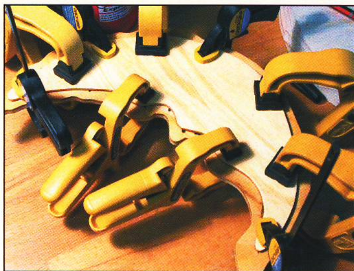
Step 20. Attach clamps to secure the pieces, and let dry. Remove any glue seepage using a toothpick or a damp cloth. Glue the overlay in place.
