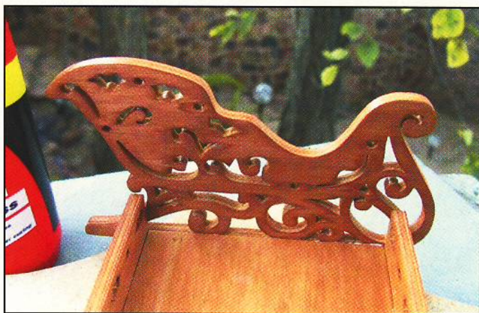
Step 15. Referring to the photograph, position the sleigh side pieces against the base assembly. The ends of the sleigh should extend evenly from both sides. When satisfied with the placement, glue the sides in place.
