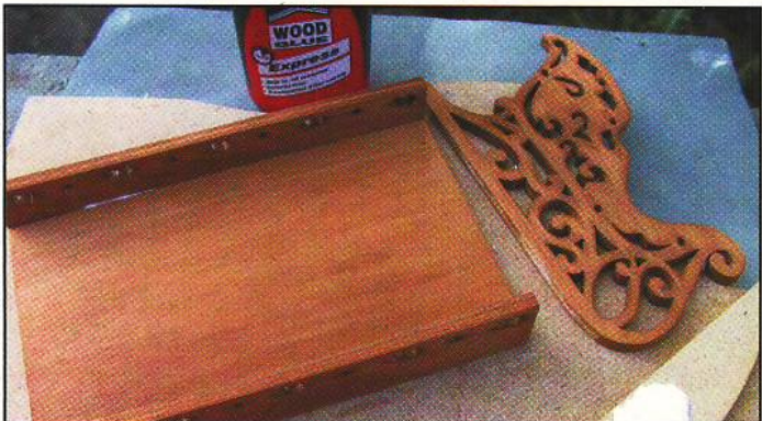
Step 14. Use wood glue to assemble the project. First, glue the front and back panels to the sides of the base. They should be flush at the ends.
