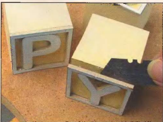
Step 10. Pry the work pieces apart by inserting a scraper blade between the layers. Remove the tape.
