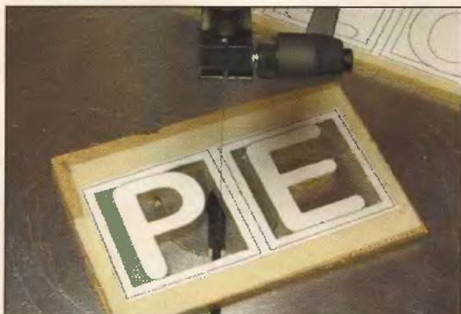
Step 6. Thread the No. 1 reverse-tooth blade through the blade entry holes, and make the inside cuts of the letters.
