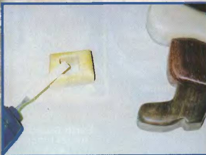
Round all the suit pieces using the oscillating spindle sander. The electro-file was very handy for sanding the inside of the belt buckle.
