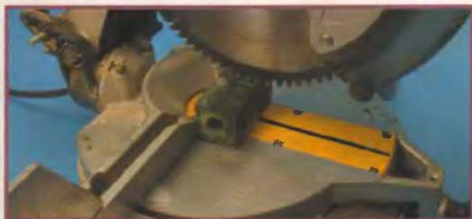
Drilled blank being cut to exactly 2-3/16" length.
