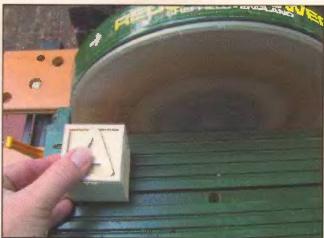
Step 9. Use the disc sander to square-sand the work pieces. Remove all patterns by peeling off the masking tape.
