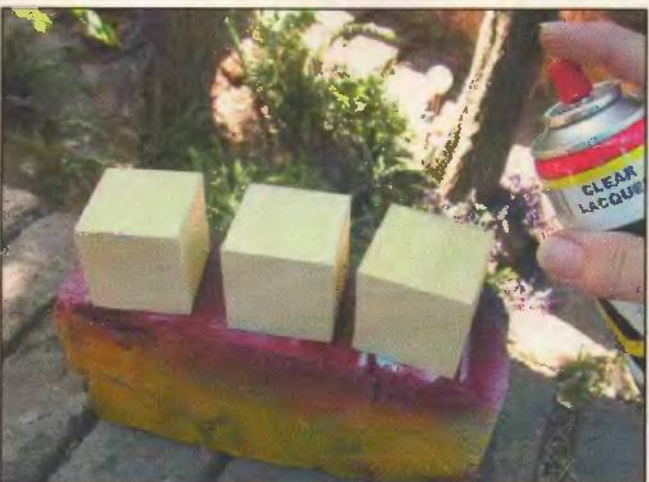
Step 13. Apply several thin coats of clear spray varnish to the blocks, letting each coat dry completely before applying the next.
