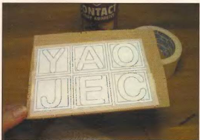
Step 4. Photocopy as many of each letter pattern as you will need for your project, saving the originals for future use. Using temporary-bond spray adhesive, attach the patterns on top of the masking tape. (If you are making more than one block of the same letter, you may want to use thin double-sided tape to join the work pieces for stack cutting, rather than cutting each letter individually.)
