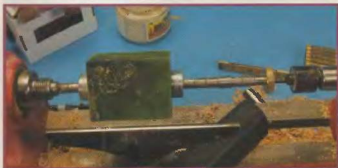
Mandrel loaded with kaleidoscope bushings, wood, and filler 7mm bushings.
