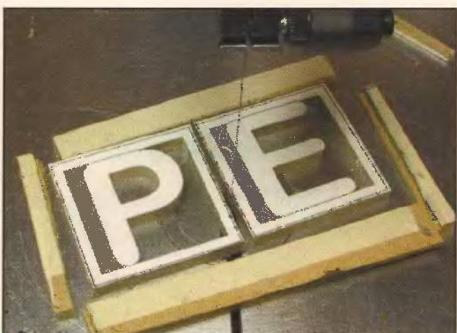
Step 7. Cut apart the squares. 1/16" beyond the pattern lines.
