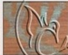
This shows the patina results after ten and thirty minutes with the drip-brush method.
