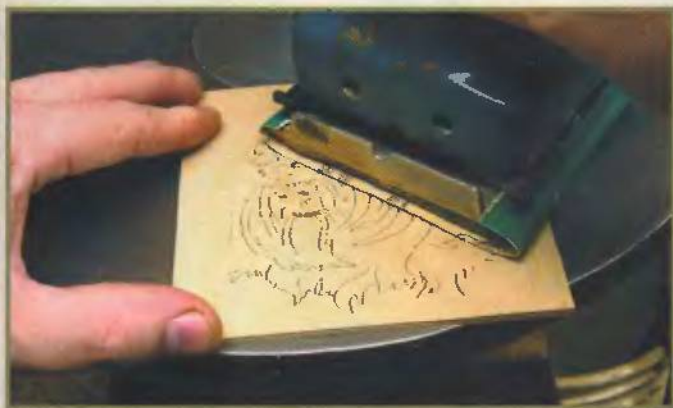
Finish sanding the back of the face.
