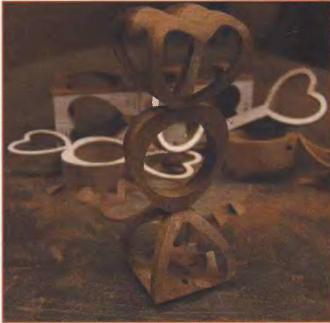
Hourglass cut and removed from waste material.
