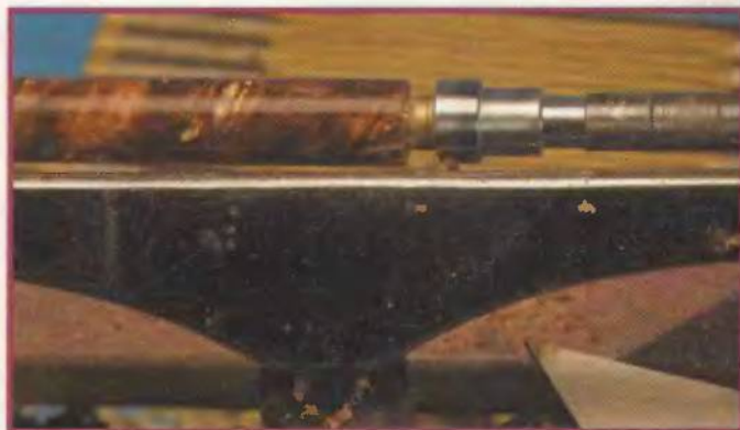
Finished and trimmed blank on mandrel with brass tube exposed. Remember: Remove the wood only to the brass tube. Do not cut the tube because it is needed for the assembly process.
