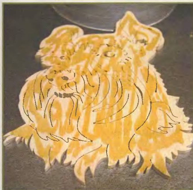
Apply CA glue to the back of the face.
