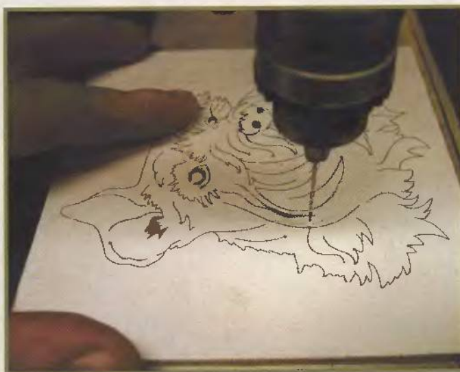
Drill at the point where the veining lines intersect.
