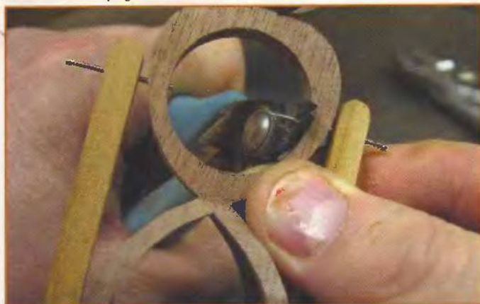
Cut off the points of the nails.
