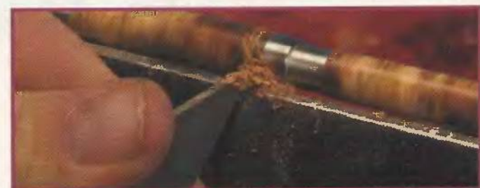
With the tool rest adjusted and the lathe on high speed, use a sharp parting tool to slowly remove the waste wood just to the brass tube.
