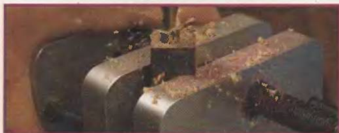
Drilling hole through blank using 8mm drill bit in drill press and with blank secured in drilling center vise.
