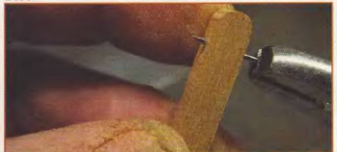
Installing a pivot pin in the yoke.
