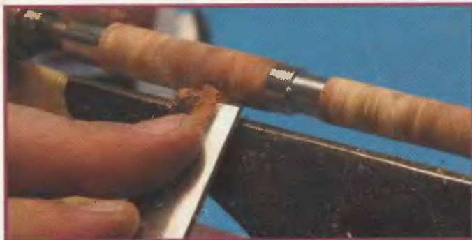
Shaping and contouring blanks using sharp skew chisel.
