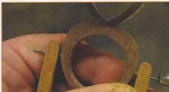
Pull the nails back through the holes.
