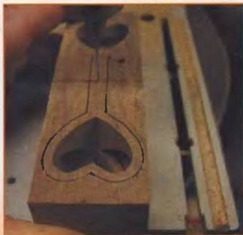
Location for drilling second pivot hole.
