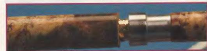
Trimmed blank with brass tube showing where trimmed.
