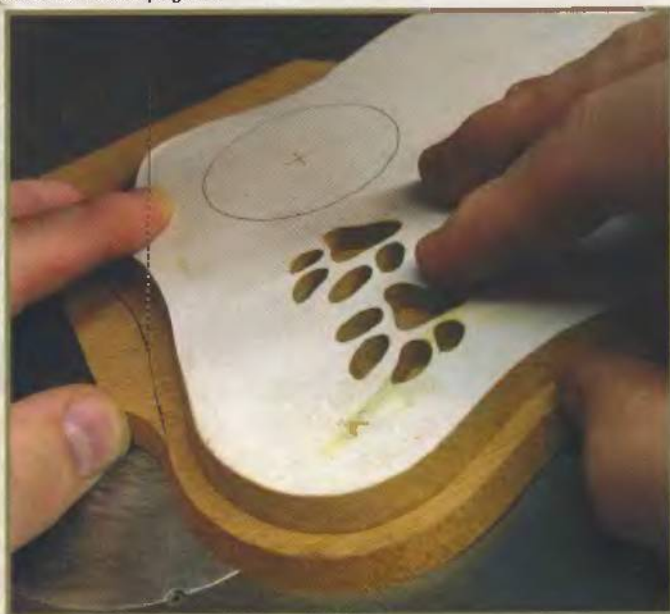
Cutting the edge of the bottom layer.
