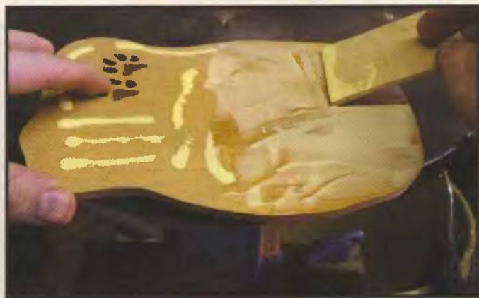
Apply glue to the back side of the cut top layer.
