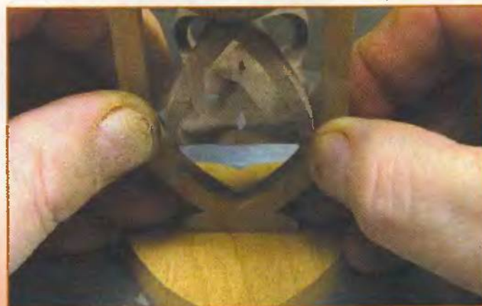
Align and glue the yoke to the base.
