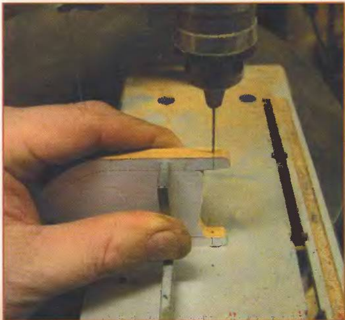
Drilling the yoke pivot holes.
