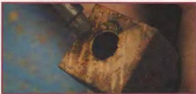
Epoxying tube into drilled blank. Push brass tube beyond any drill damage.
