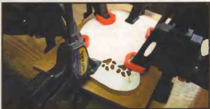
Clamp the cut top layer to the wood for the bottom layer.
