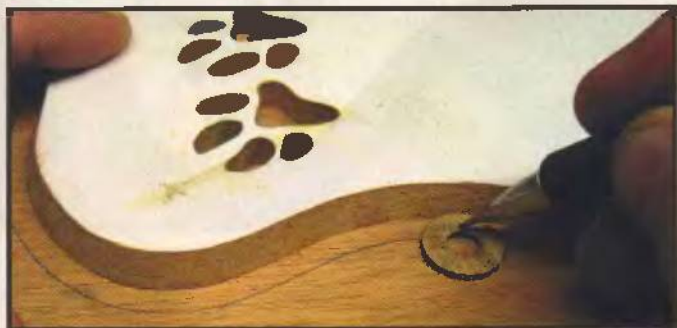
Use a washer or circle template to trace the pattern line for the bottom layer.
