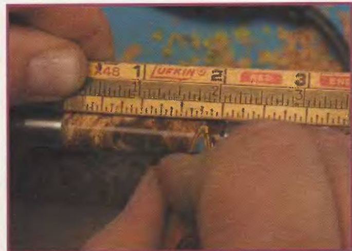
With the pen blank still on the mandrel, measure and mark the cap tube at 1-13/16" all the way around.
