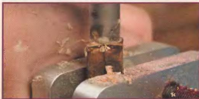
Square and true both ends of each blank using the 8mm barrel trimmer, with the blank mounted in the drilling center vise.
