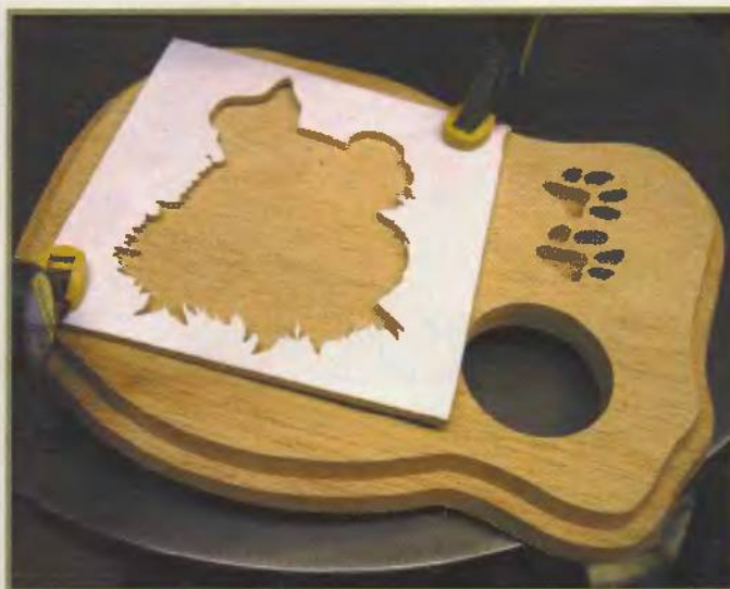
Clamp the waste piece to the backer.
