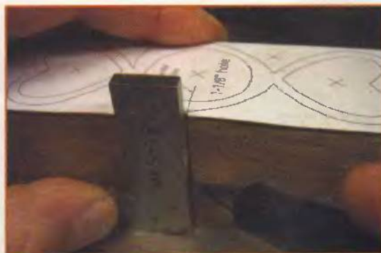
Use the pattern transfer line and a square to draw a line down the side of the wood.
