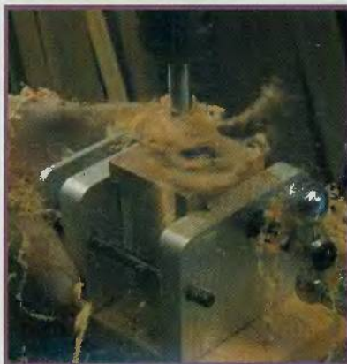
Drill center hole in blank using 1-3/8" forstner bit in drill press.
