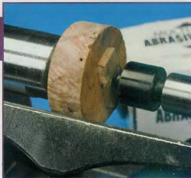
Mounted blank in lathe with tail stock and scrap wood.
