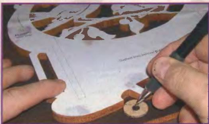
Drawing the pattern line for the backer board.
