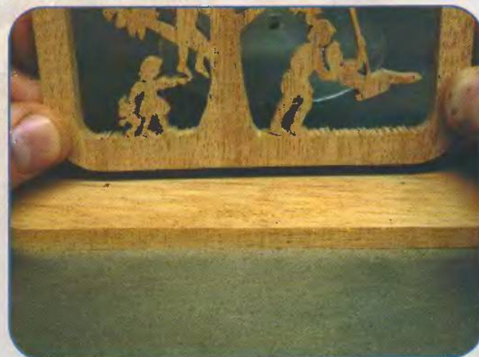
Aligning and gluing the tree swing to the base.
