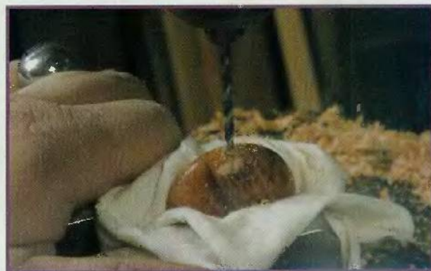
Secure cloth-wrapped blank in drilling center vise and drill 3/16"-deep hole with 9/64" bit mounted in drill press.
