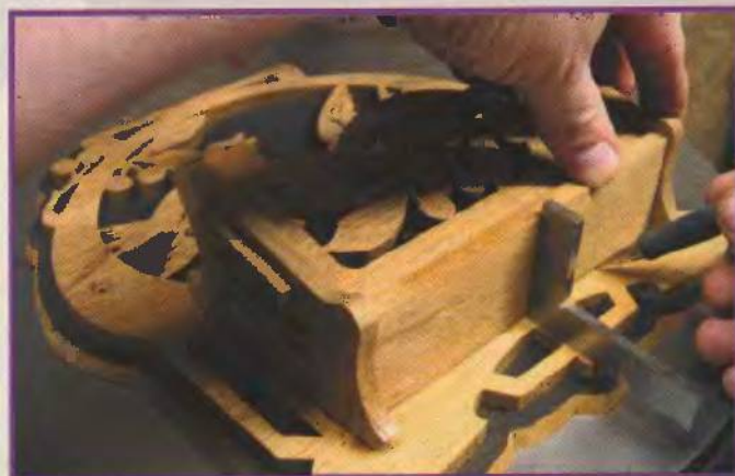
Pocket parts held in place while marking position of bottom piece.
