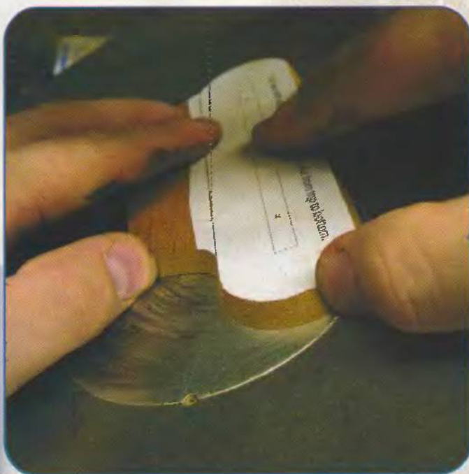
Cutting beveled edge of base.
