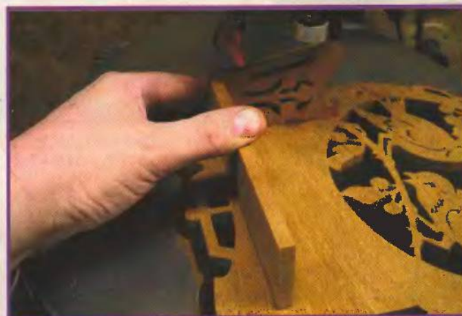
Gluing on the bottom piece of the pocket.
