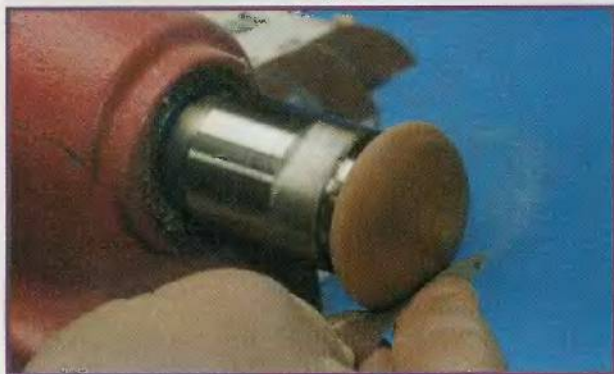
Start sanding using 150-grit cloth-backed sandpaper and the lathe on low speed.
