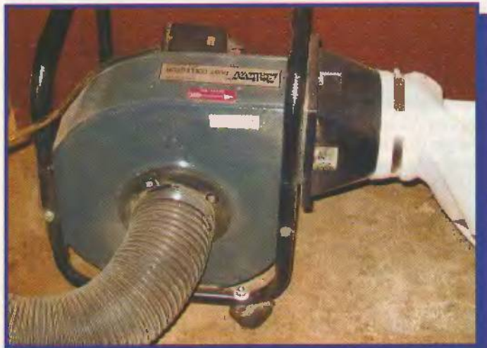
A dust collection system with a 4" intake hose, positioned as close as practical to the sanding drum, is also an efficient arrangement for edge sanding and contouring.
