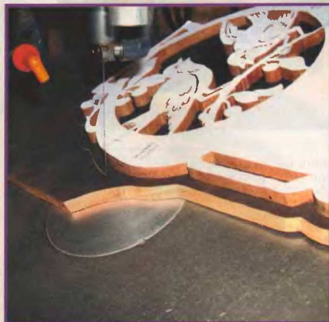
Cutting the backer board.
