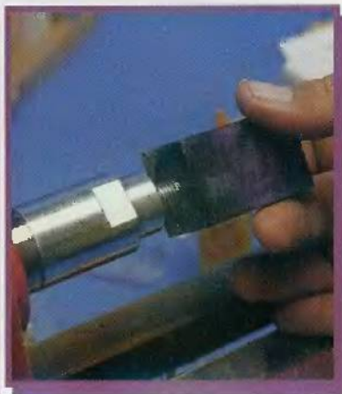
Fig. 4. Mounting the blank on the mandrel.
