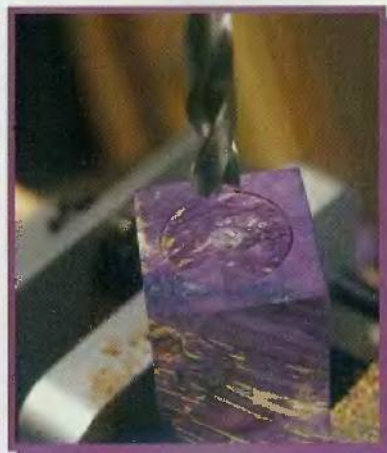
Fig. 2. Insert the 23/64" bit in the drill press. Note the position of the drill does not change.
