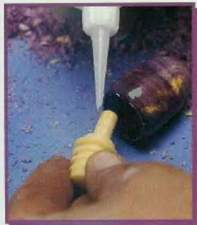
Fig. 11. Place a drop or two of instant glue inside the turning, then screw the chrome stopper into the wood.
