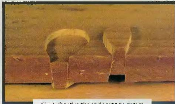
Fig. 4. Practice the angle cuts to ensure that the wood rotation is correct.
