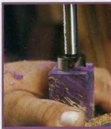
Fig. 1. Place the blank in the centering drill vise with the 1" forstner bit in the drill press.
