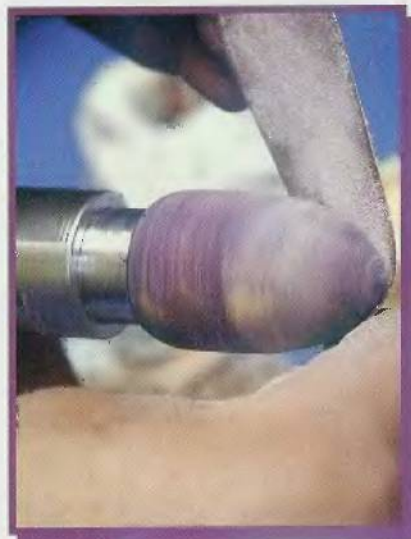
Fig. 7. Frequently stop the lathe to check the surface condition as you sand your turning.
