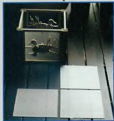
Fig. 11. Glue the Lexan piece flat against the maple panel.
