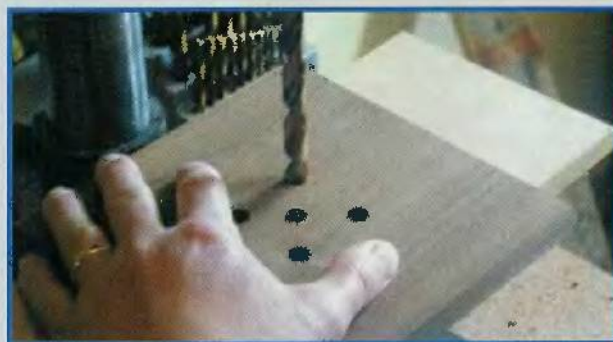
Fig. 8. Drill the light kit and venting holes in the base.
