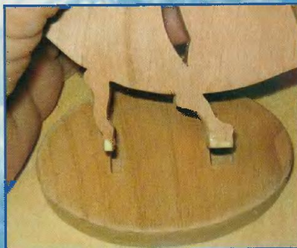
Step 9. Apply wood glue to the tabs at the bottom of the angel. Insert firmly into the base. Wipe off any excess glue with a damp cloth. Apply several coats of a clear finish of choice and let dry. Press the clock insert into place.
