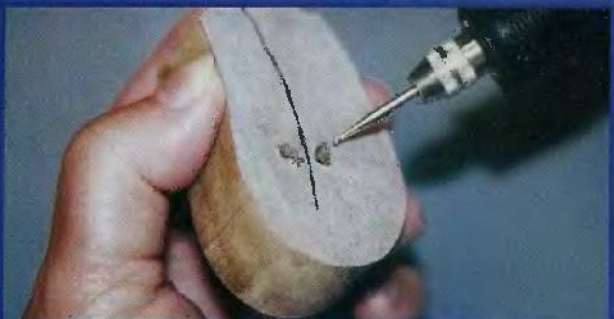
Fig. 9. Clean up drilled holes
