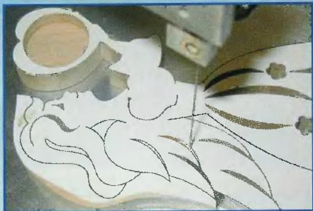
Step 5. Cut around the outside lines of the angel and base.
