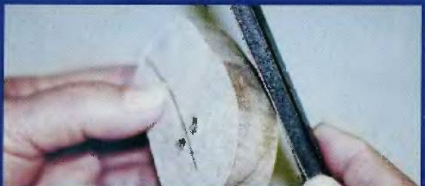
Fig. 6. Deburr back edges of cut piece
