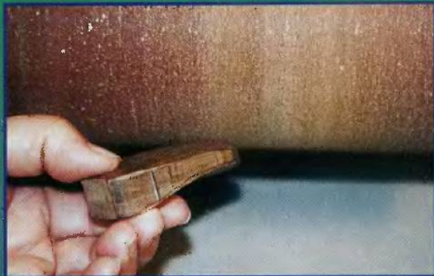
Fig. 13. Contour the duck-bill on both sides
