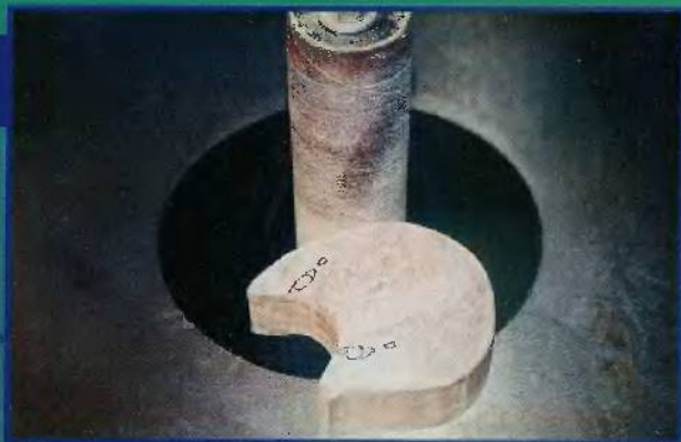
Fig. 7. Ensure a 90° angle on the cut
