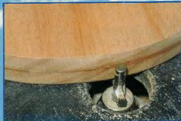
Step 7. (Optional) Using a 1/8" round-over bit installed in a rotary tool, round over the top edge of the base.
