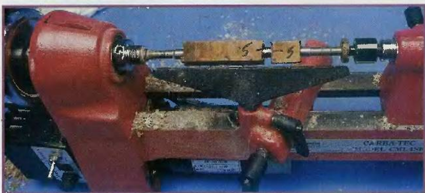
Fig. 3. Load the mandrel with the applicator blanks
