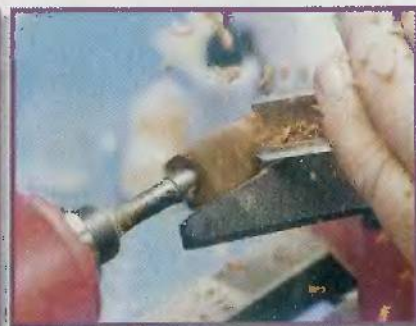
Fig. 4. Use your rough-out gouge to round out the blanks
