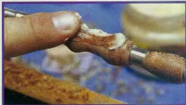
Fig. 7. Apply Shellawax Cream while the applicator is on the lathe
