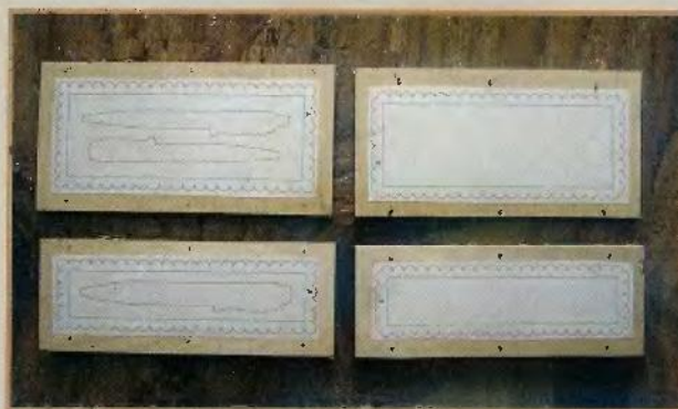
Nailed stacks ready to cut. I traced the outlines of the pens and pencils I was using to create the patterns for the cavities.
