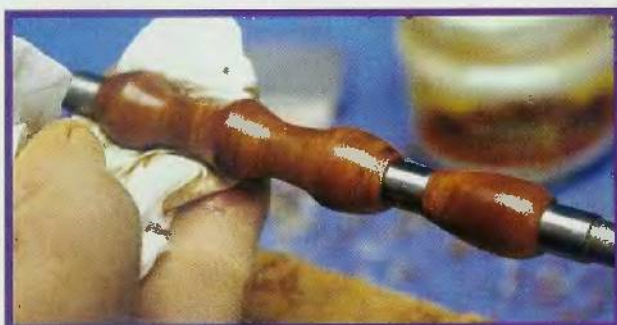
Fig. 8. Begin buffing with the lathe on medium speed, and move quickly to high speed for a nice shine
