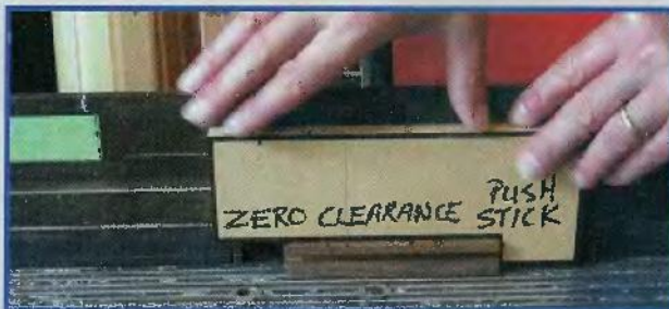
Fig. 1. Run all four posts over the blade using a safe push stick.
