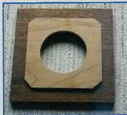
Fig. 12. This shows the walnut lid with the attached maple underside panel. The center hole is the opening for the glass chimney.
