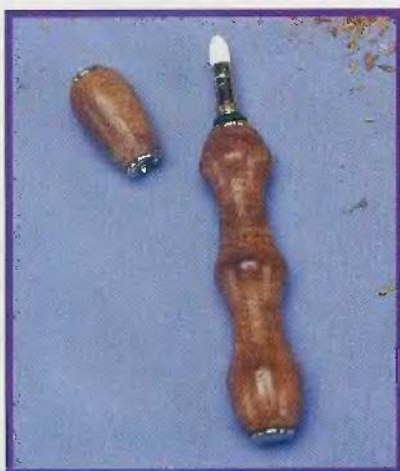
Fig. 8. Begin buffing with the lathe on medium speed, and move quickly to high speed for a nice shine
