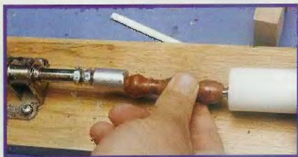
Fig. 9. The pen press is a handy helper for the assembly process
