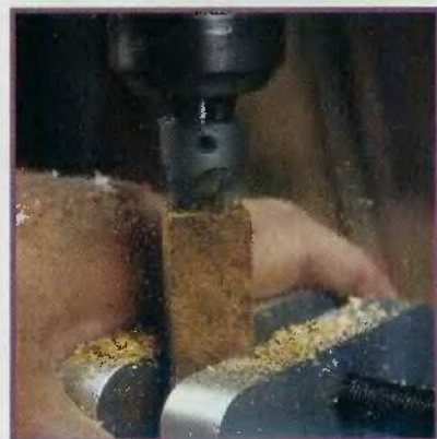
Fig. 2. Use a barrel trimmer with tape wrapped around the 7mm shaft
