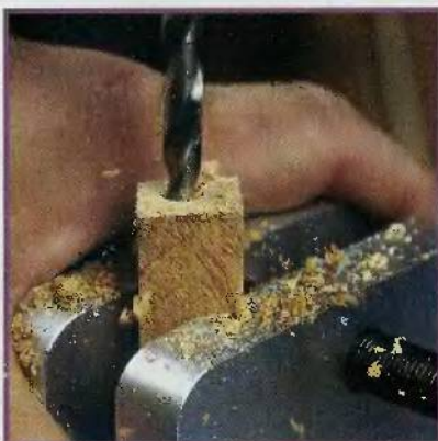
Fig. 1. Drilling with the blank in the vise
