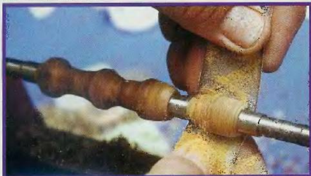
Fig. 6. Sanding the pieces on the lathe
