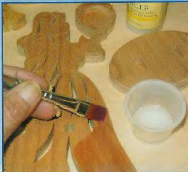
Step 8. Remove the patterns from the wood. Sand the pieces smooth, then apply a coat of wood sealer. Allow to dry, then sand smooth again with 400-grit sandpaper.
