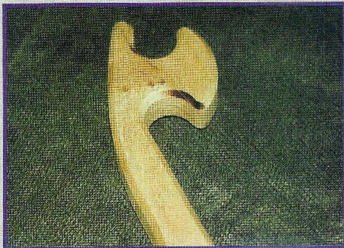
Fig. 8. Small burn marks such as these are almost unavoidable when using cherry; they are very difficult to remove with abrasive paper alone!
