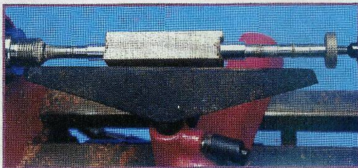
Fig. 3. Install the mandrel on the lathe.
