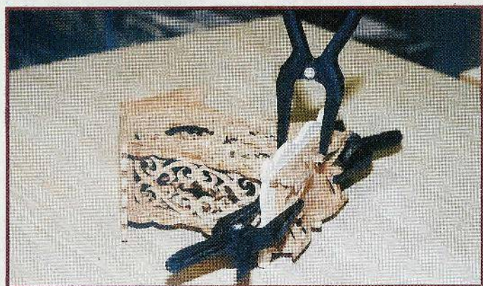
Fig. 2. Glue the body assembly to the foot assembly.
