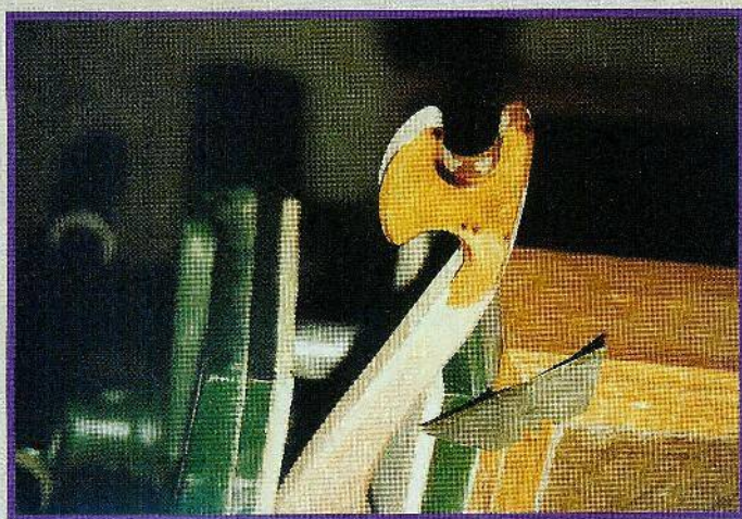
Fig. 9. I flood the surface with either linseed oil or paint thinner and then use the blade from a utility knife as a scraper to remove the burns.
