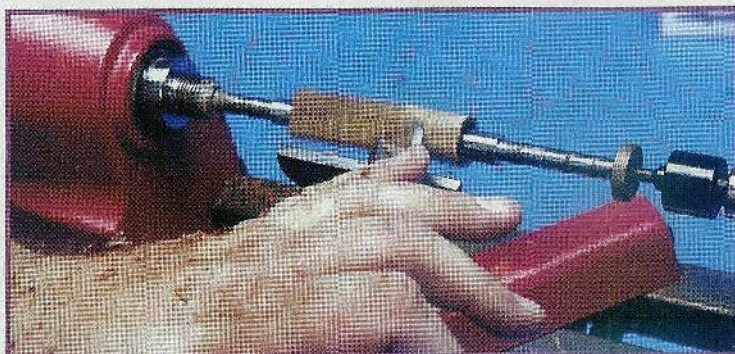
Fig. 4. With a roughout gouge, begin to round the pen at low speed using a slow straight cut down the length of the pen
