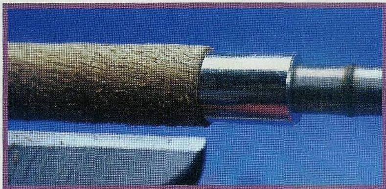
Fig. 5. A close-up of the turning before being sanded.
