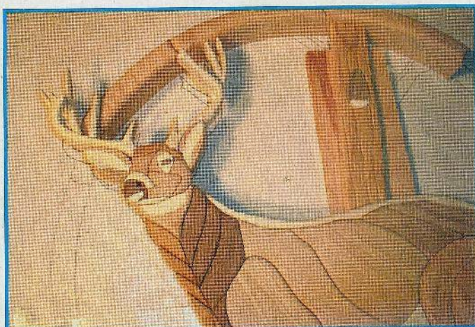
Fig. 25. Glue the frame assembly to itself and to the buck, snow, and tree as you go.
