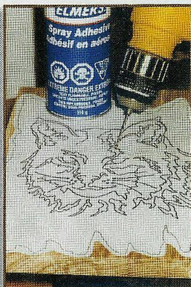
Fig. 1. Drill starter holes in the waste areas to be cut out.
