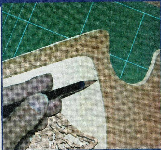
Step 10. Mark the placement of the plaque on the backer board and the moon on the upper right corner of the plaque.
