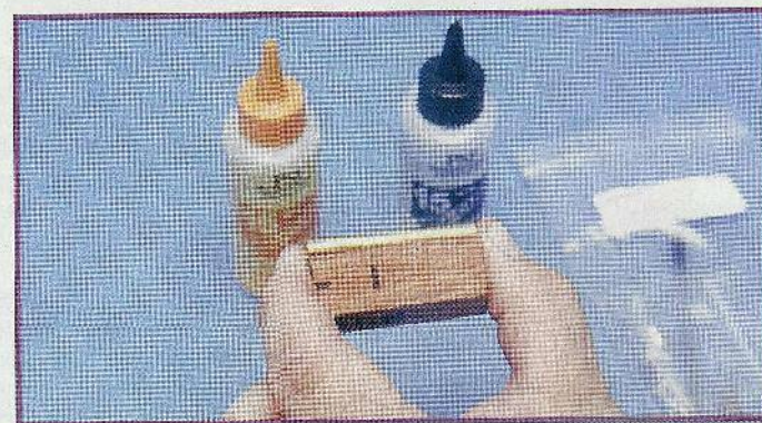
Fig. 3. Use two-part liquid epoxy to glue in the brass tube.
