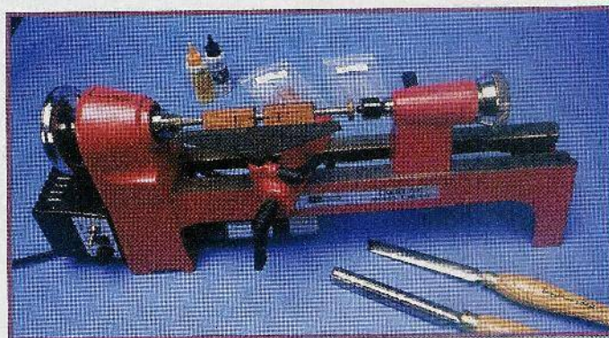
Fig. 6. Follow the kit instructions for loading the mandrel.
