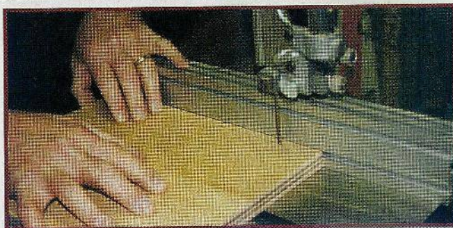
Fig. 5. Removing the rest of the scrap in the notch is easier and more accurate if you use a fence on your hand saw. However, if your blade is too dull, it will sometimes lead to the dull side and create problems.
