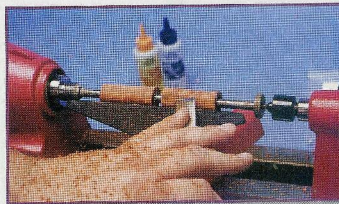
Fig. 7. Use a gouge to turn down your blanks.
