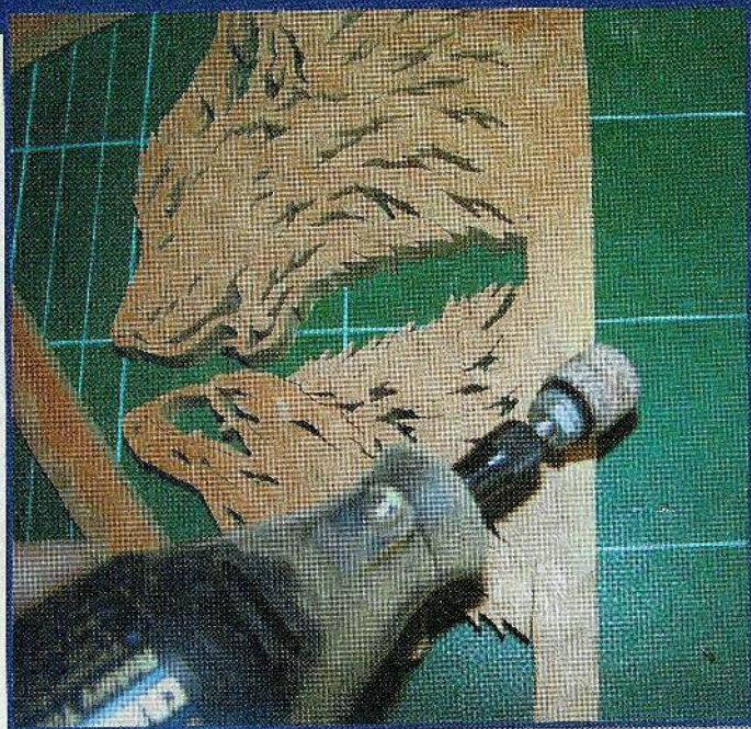
Step 7. Use the rotary tool to round the edges of the plaque randomly so that it resembles a carved arrowhead.
