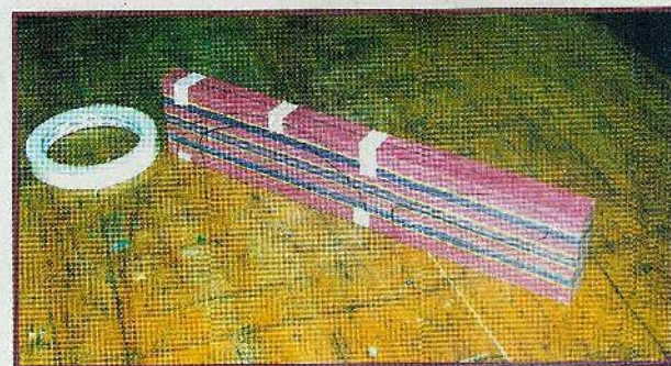
Fig. 4. When the cuts have been made, I used 1/2" masking tape to reattach the pieces of scrap to where they were originally located on the blank.
