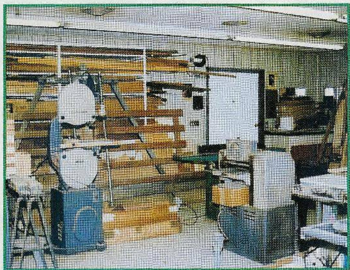
Fig. 8. Ira uses many shop-built tools and assembly jigs; note the shop-built panel saw "hiding" behind the band saw.
