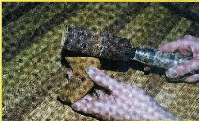
Fig. 4. I like to use a small pneumatic sander called the "Sandstorm Sander" to shape down to the guide lines.
