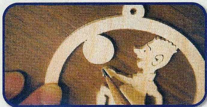
Fig. 6. Small imperfections can usually be sanded out.
