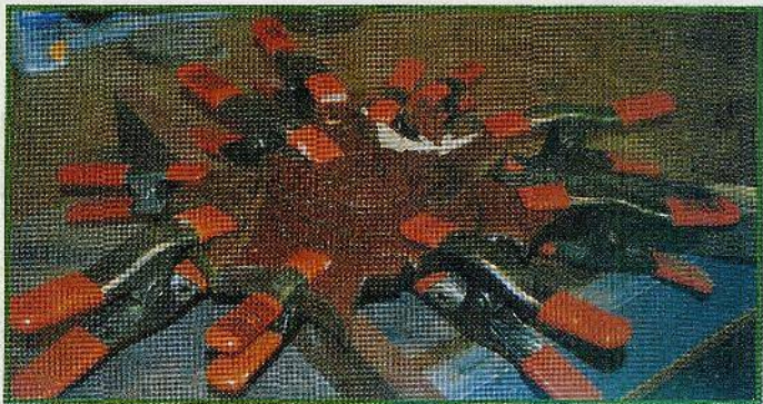
Fig. 10. Glue the assembled project onto the backer board and clamp in place.
