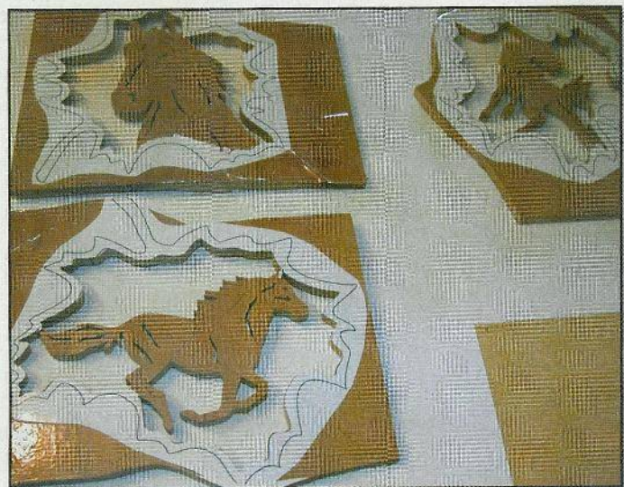
Fig. 3. Attach the sheet of Baltic birch to the back side of your cut-out patterns.
