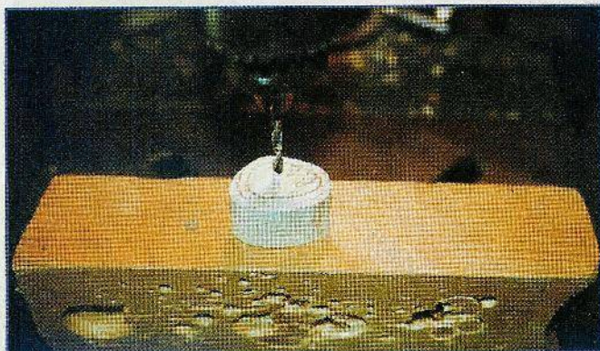
Fig. 6. Drill out the middle of the eye pattern on the butternut using the drill and an appropriately sized bit, and then cut, sand and deburr as with the other pieces.
