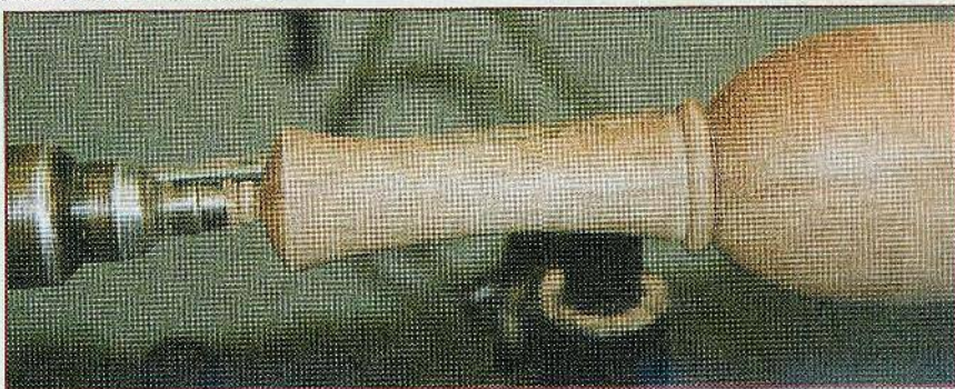
Fig. 9. The shape of the handle has been turned and the bead detail is defined.
