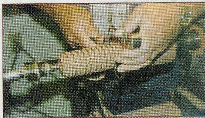
Fig. 3. A series of cuts are made with the parting tool on the remainder of the stock, spaced approximately 3/8" to 1/2" apart.
