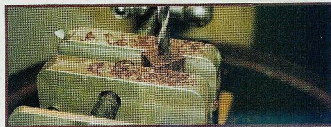
Fig. 3. Find the center of both blanks and drill them using the pen drilling vise. Be sure to drill the ends marked with the "X."
