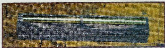
Fig. 1. Start by laying the tubes directly on the blank.
