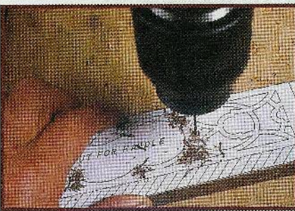
Step 6. Apply the patterns to the appropriate surfaces with spray adhesive. Drill the blade entry holes with a drill bit that will accommodate your blade.
