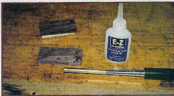
Fig. 5. Use the pen tube insertion tool and thick superglue to secure the tubes in the blank. Be sure to position the tubes from the end with the "X."
