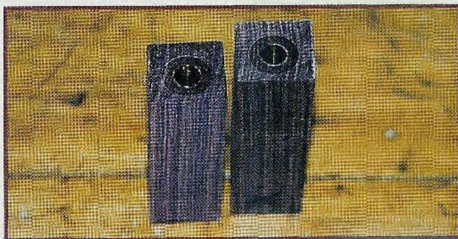
Fig. 6. Use the barrel trimming tool to square up the tubes with the wood.
