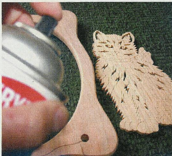
Fig. 10. Spraying the backer board, kitten and frame with several coats of varnish.
