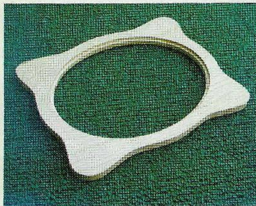
Fig. 5. The frame's back inner edge has been rabbeted.
