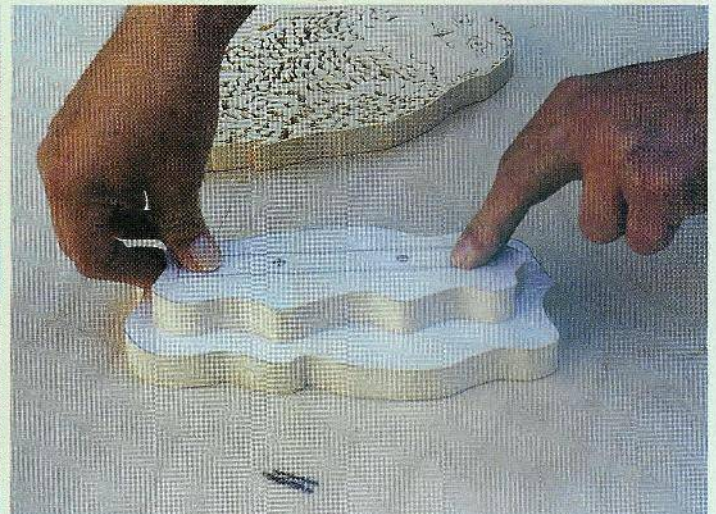
Fig. 1. Marking for guide holes on the bottom of the smaller base piece with finishing nails placed through the 1/16" holes in the larger base piece.
