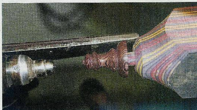
Fig. 6. Oops! The turning separated where it wasn't supposed to. I liked the look, however, and decided to keep it.
