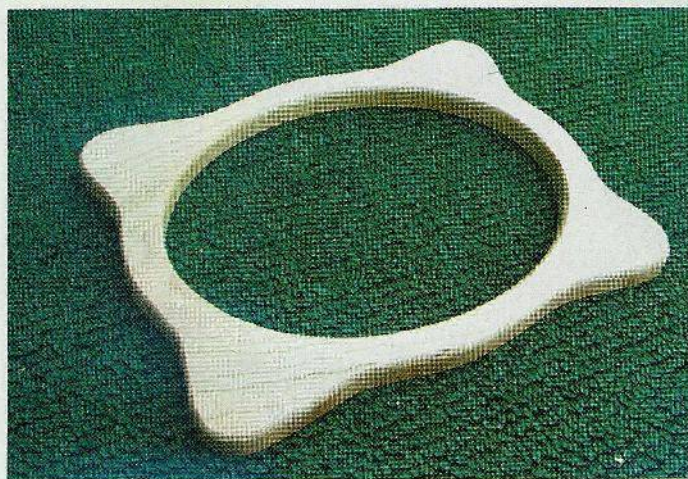
Fig. 3. The frame's inner and outer edges have now been rounded over.
