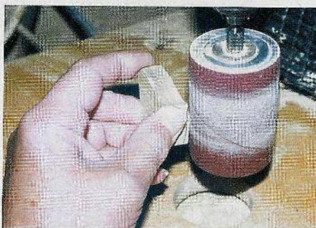
Fig. 25. Sand the parts to the contour line.
