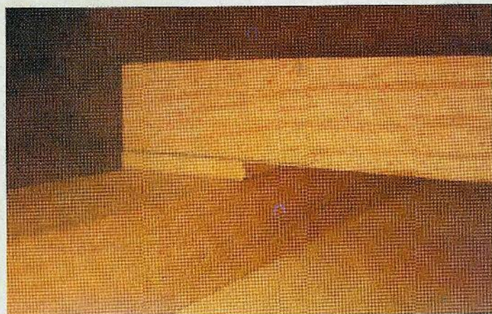
Fig. 2. 1/8" spacer to raise guide pin strip for clearance.
