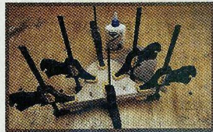
Step 10. Glue the layers together using a glue of your choice. Do not attempt to apply glue to all of the layers and then assemble and clamp. The glue applied first will begin to dry before you can apply it to the other layers, and that could present bonding problems. Use plenty of clamps to insure good adhesion.
