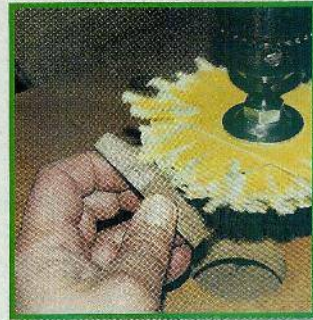
Fig. 18. A sanding mop is used to smooth the pieces.
