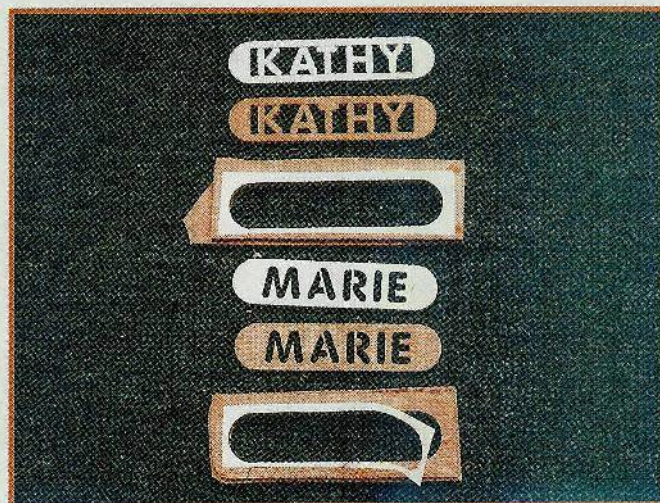
Fig. 4. Saw around the perimeter of the pattern.
