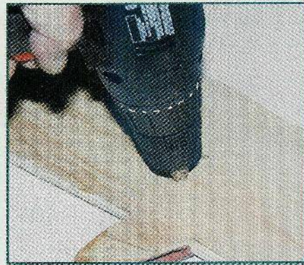
Fig. 19. Countersink for the screws which will secure the rod holder dowels.
