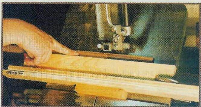
Fig. 2. Rip the 45 degree bevel on the trim piece.
