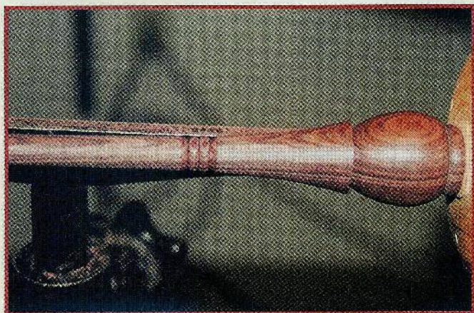
The two decorative beads have been turned in the middle of the handle. Note the transition shapes that visually connect the two small beads to the rest of the turning.
