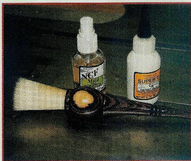
The duster is complete and the finish has been buffed to a shine. I glued the bristle head in with super glue. An accelerator made specifically for this brand of glue was used to speed up the bonding process.
