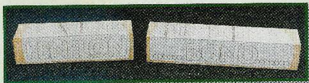
Center the patterns on the square stock and bore blade entry holes as needed to prepare for sawing. Cut the open letters first.
