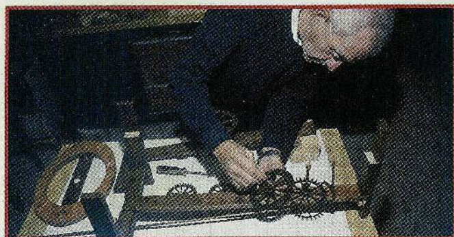
Assembling the works. All finish is applied and allowed to cure several days before assembling.
