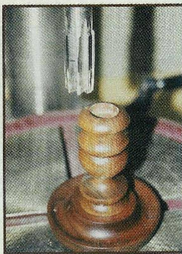
I use a reamer to establish the taper that matches the base of the wax candle.
