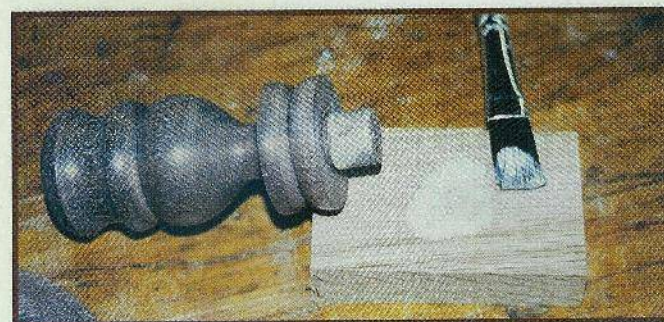
Glue is applied to the tenon with a brush. I only glue the tenon because end grain doesn't stick well to surface grain and because I don't want glue flowing out of the joint.
