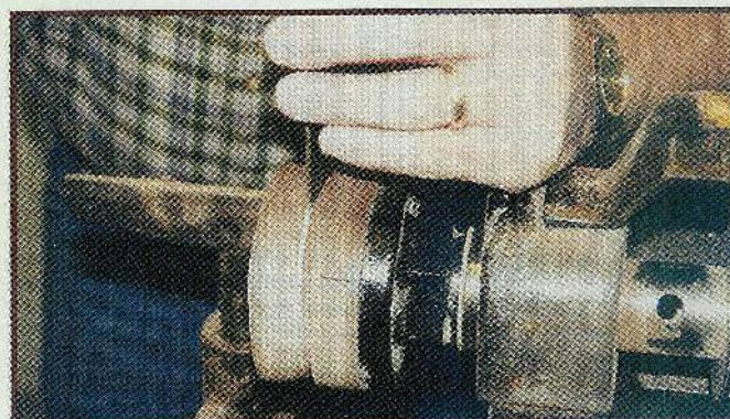
A sharp chisel with a wide blade is used to break the joint apart. Place the flat side of the chisel against the side you wish to keep and tap it sharply with a mallet. It should come apart easily.
