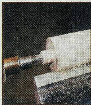
The spindle is mounted between centers ready to turn. Note the small spur center used in the headstock end of the lathe. This allows the tenon to be turned without interference.
