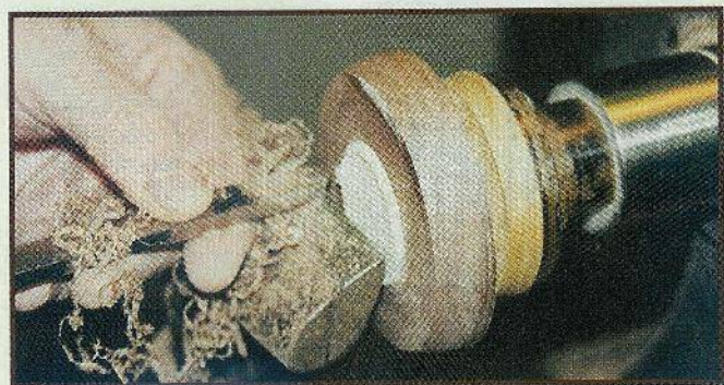
The paper is removed and the base is undercut about 1/8" to 3/16" to form a stable ring. Turnings stand better on a ring rather than on a flat base.
