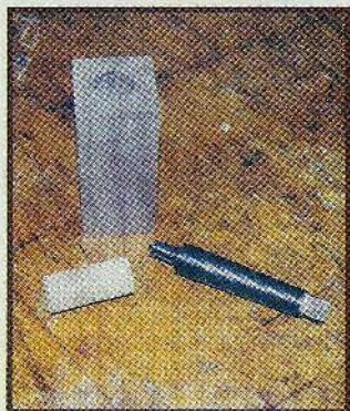
I turned a plug to fill the hole I had just drilled so that I could mount the spindle between the centers and turn it to the proper profile.
