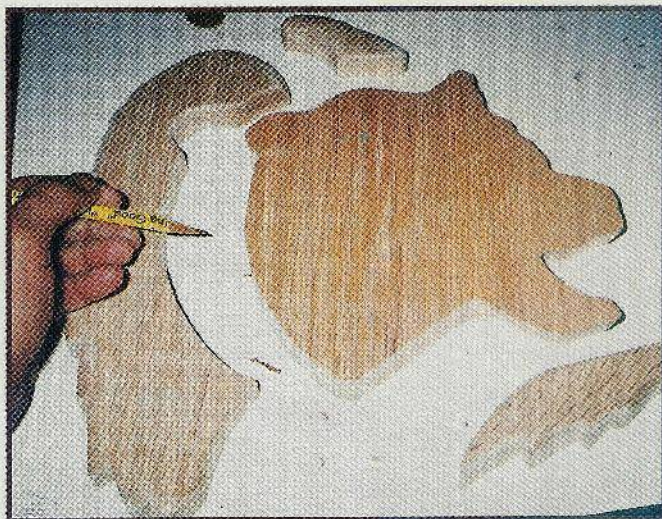
Step 8. Cut and fit the shoulder pieces, including the piece which will be beneath the head piece. Hint: this piece can be made out of plywood instead of oak as shown here. Round over the pieces, stain and edge glue them together. Finally, glue the head piece in place on the shoulder piece.
