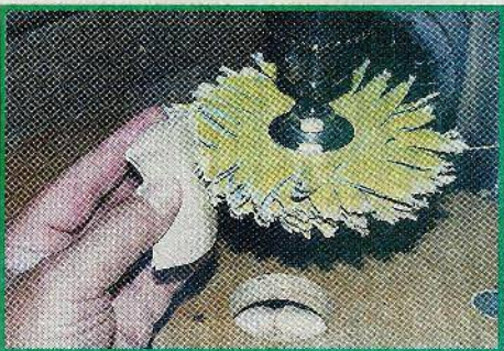
Fig. 9. Smooth each piece with the sanding mop.
