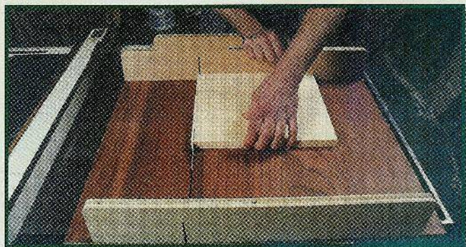
Fig. 1. A sliding cross cut table is used to accurately square off the first end of the side piece. A regular miter gauge can also be used.
