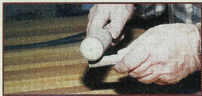
Fig. 4. Shape the pieces. I like using a pneumatic drum sander in a flex shaft tool for this operation.
