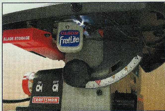
Fig 2. The switch can be mounted in the leading edge of the table or at any other location you desire within the limitations of the length of the switch wire.
