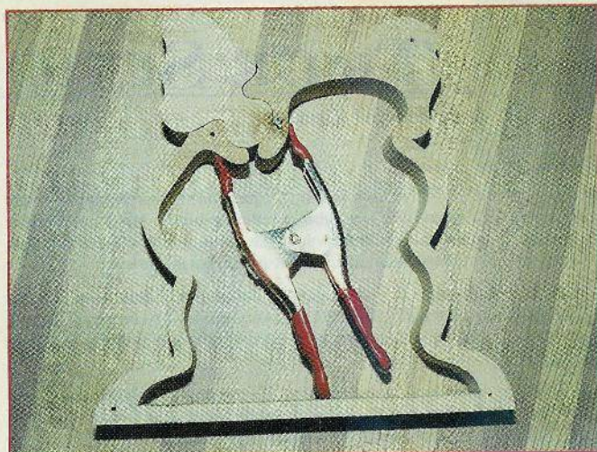
Fig. 4. Be careful that the slot for putting money into the bank does not spread. Put the ear in place and use a spring clamp to keep it from spreading.
