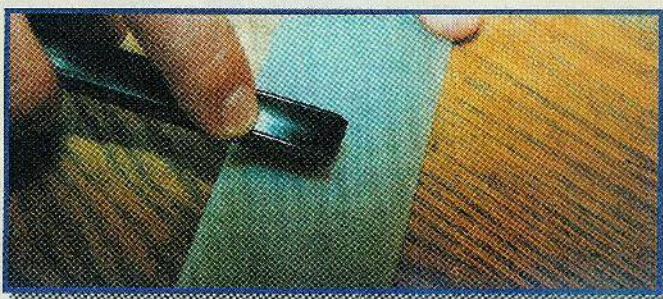
Fig. 6. Shape the bottom of the V as if it were a gouge.
