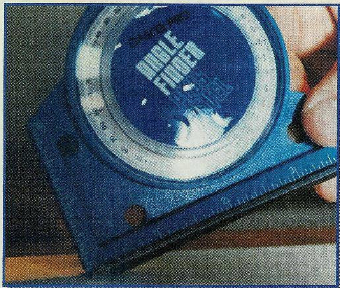
Fig. 1. It is important to get the right bevel on your carving tools. I grind my tools to a 20 to 25 degree angle.
