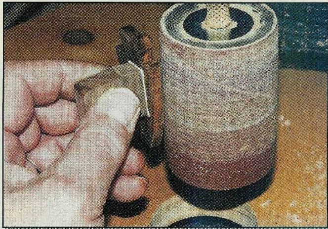
Fig. 2. Use a drum sander to shape the piece.
