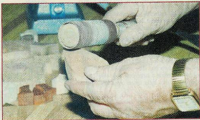
Fig. 1. I use small pneumatic sanding drums to shape my intarsia pieces.
