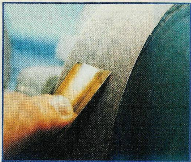
Fig. 2. Try to avoid a hollow ground bevel which will result by holding the tool square with the wheel.
