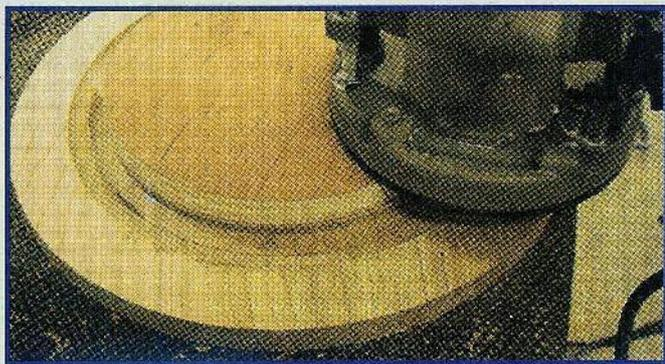
Fig. 6. Routing the groove in the top.
