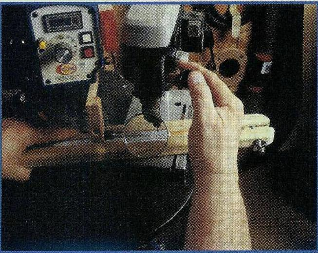
Fig. 4. John uses a mini-drill press on his scroll saw's table, thus getting the use of its magnifier and light.
