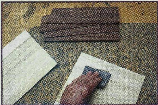
**Step 1.** Sand all pieces to 220-grit and remove any mill marks or surface blemishes.
