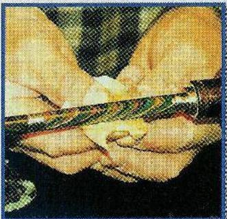
Fig. 15: A liberal coat of a Danish oil brings out the beauty of the wood. I use toilet paper to apply the oil and to remove any excess.
