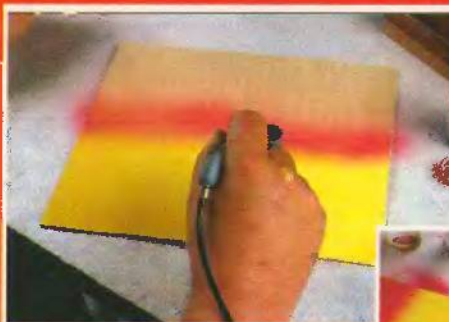
Fig. 2. Using an airbrush gives you more control over the amount of paint applied. Just make sure you keep it clean!
