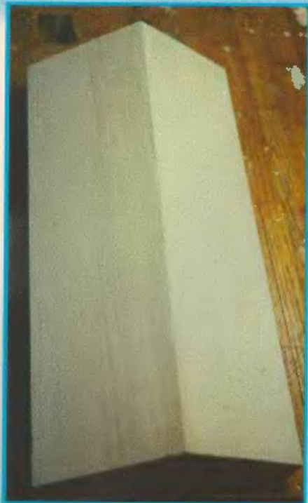
Fig. 1. Cut a 30 degree angle in the wide side of the wood stock.
