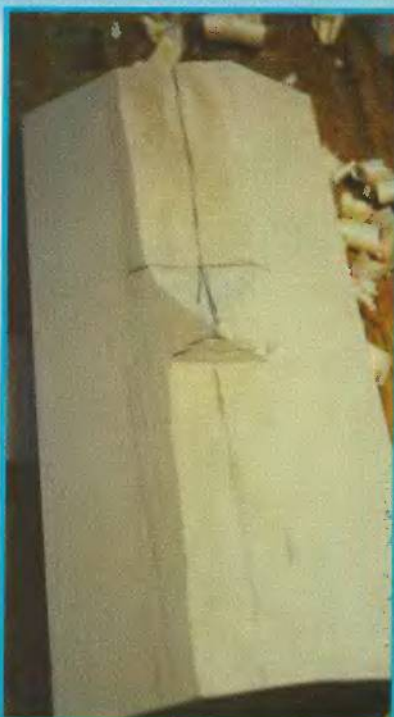
Fig. 2. Make stop cuts above and below the nose. Remove stock to the top and bottom of the board.
