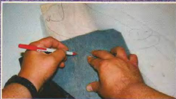
Fig. 1. Transfer the pattern to the wood.
