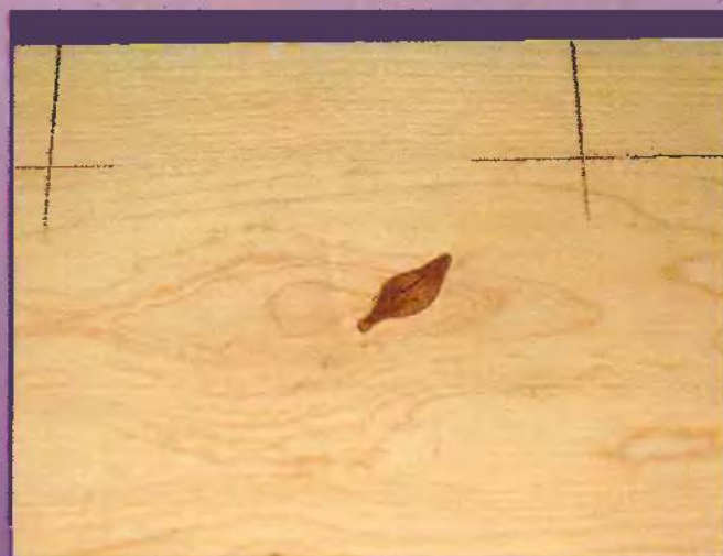
Fig. 4. Glue the inlay piece in place.
