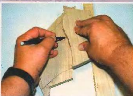
Fig. 4. Use the sanded edge as a template to trace a new, accurate cut line on the adjoining piece.
