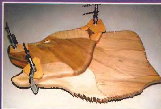
Fig. 16. Clamp the pieces together with C-clamps.
