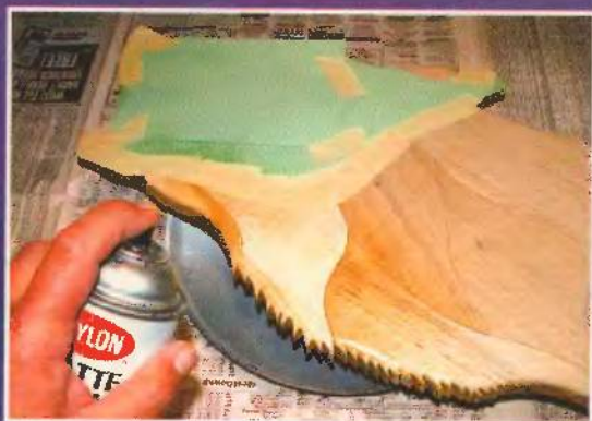
Fig. 15. Before applying the finish, mask the plywood backer with tape and paper to insure a good glue bond.
