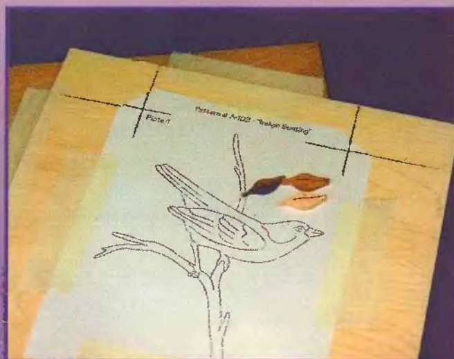
Fig. 3. Discard the waste piece from the panel and keep the inlay piece.
