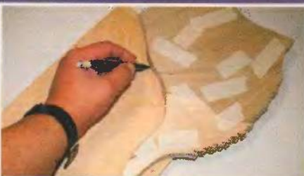
Fig. 7. Trace the edge of the neck unit onto the backer.
