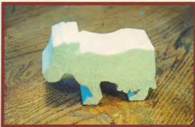
Fig. 1. Cut away the waste wood to block out the pattern.
