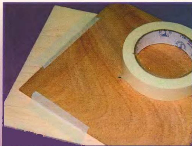
Fig. 2. Attach the inlay piece to the underside of the panel.
