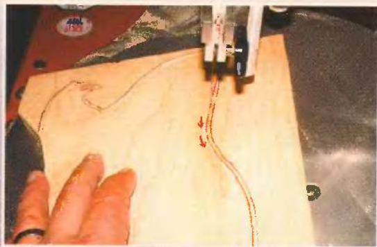
Fig. 9. Tilt your saw table 15 degrees left and cut approximately 1/8" inboard of the traced line.
