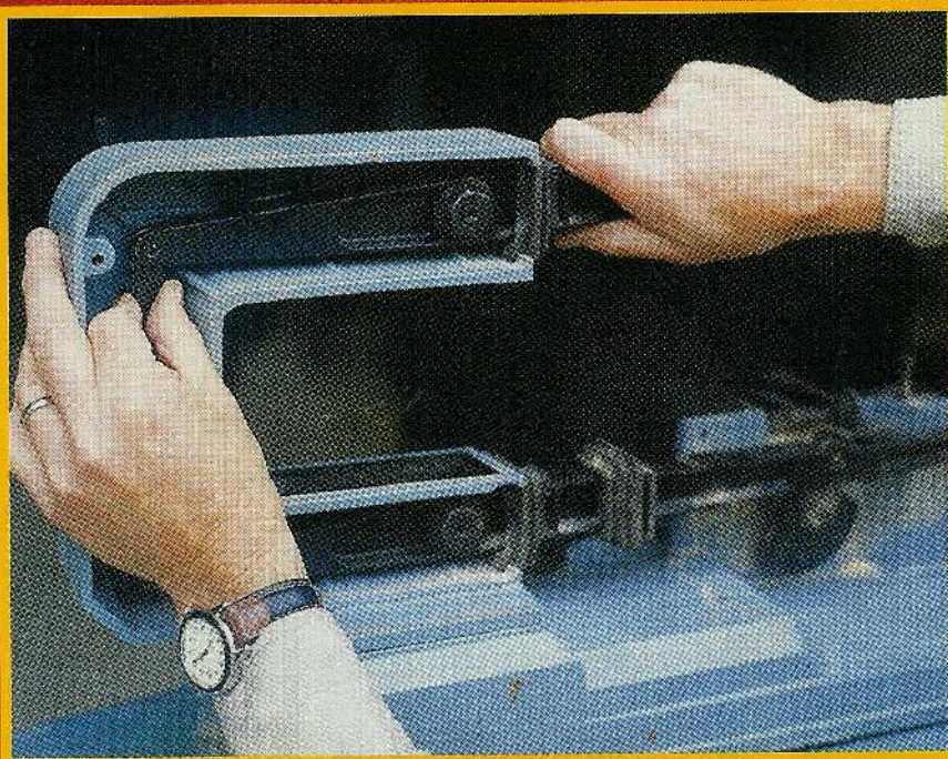
Fig. 1. The drive line is where rotational motion is converted into linear motion. Any place where the direction of motion changes is subject to wear.
