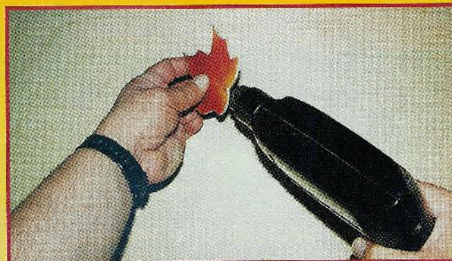
Fig. 3. Drill a hole for the stem with a No. 60 bit.
