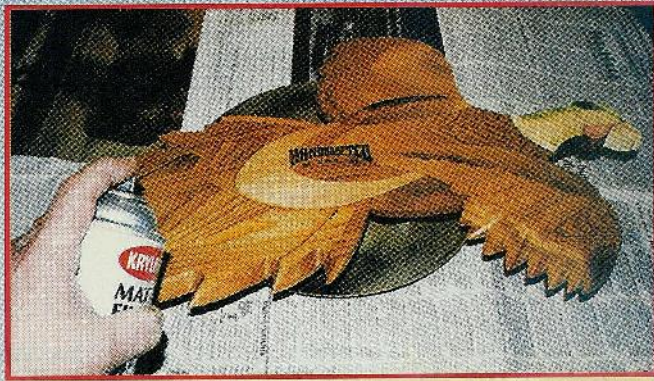
Fig. 11. Using a turntable makes easy work of finishing your project evenly and completely.
