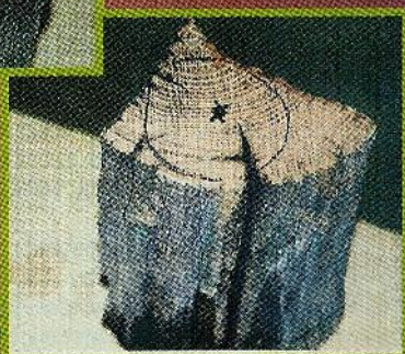
Fig. 5. Drilling out the initial hole with a 3/8"-Dia. brad point drill bit to a depth of 2-1/2"
