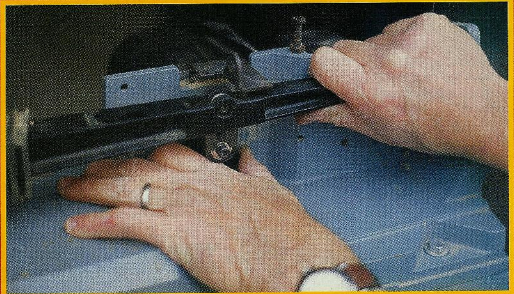
Fig. 4. Check the connecting rod as well as the drive shaft. If you feel any play or see lubricant squeeze out, it's time to rebuild.
