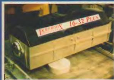
Alabaster can be surfaced just like wood. My Performax drum sander worked great for this purpose.
