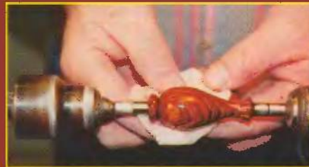
Fig. 15. Applying the Mark II oil to the turning.
