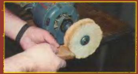
Fig. 16. Loading the Tripoli wheel to start the buffing process.
