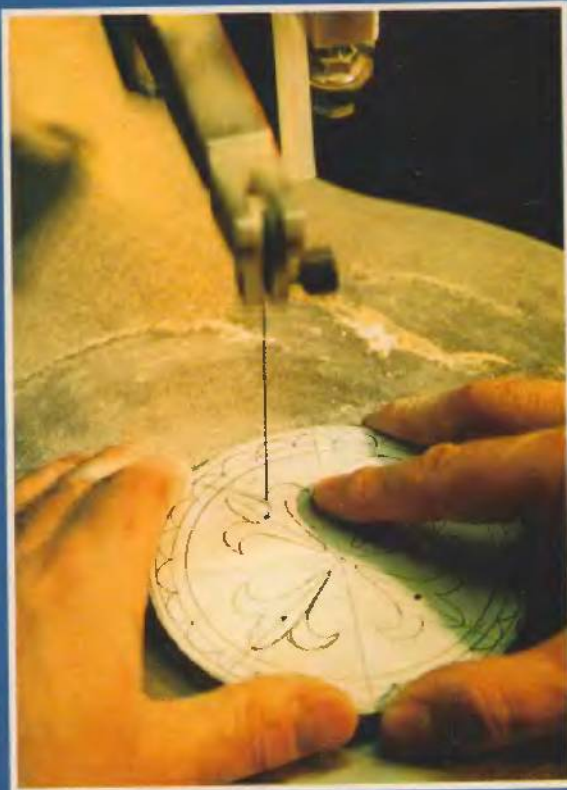
Fig. 1. Bore blade entry holes in the waste areas and make the interior cuts first.
