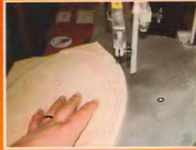
Fig. 3. Tilt your saw table 15 degrees to the left and cut out the backer board 1/4" in from the outline of the plaque.
