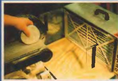
Alabaster can also be finished with conventional woodworking tools. Shown here is an alabaster disc being smoothed with a belt sander.
