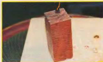
Fig. 3. Drilling out the center with the brad point bit. Either a regular 7mm brad point drill bit can be used or a 1/4"-Dia. "bullet drill" bit made by Black and Decker. Personally, I prefer the latter because it seems to drill a straighter hole. This bit is available from most home centers or from HUT Products for Wood.
