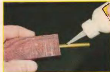
Fig. 4. Applying glue to the brass tube. Be sure to use enough to do the job!
