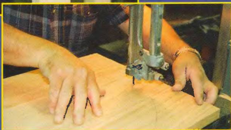
Fig. 8. Cutting out the top on the band saw using a circle cutting jig.
