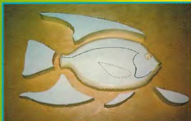
Fig. 2. Cut the outer parts, then rout the body edges.
