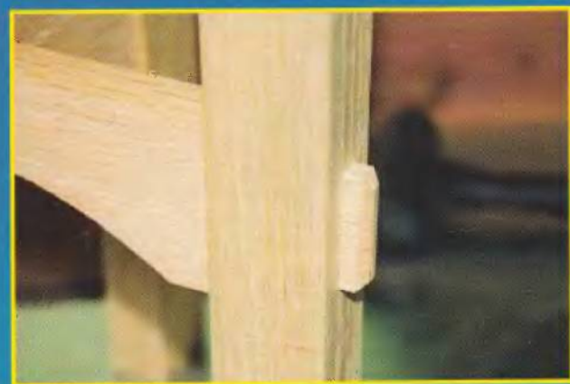
Fig. 6. The lower rail. Decorative chamfers have been cut on the ends of the exposed tenons.
