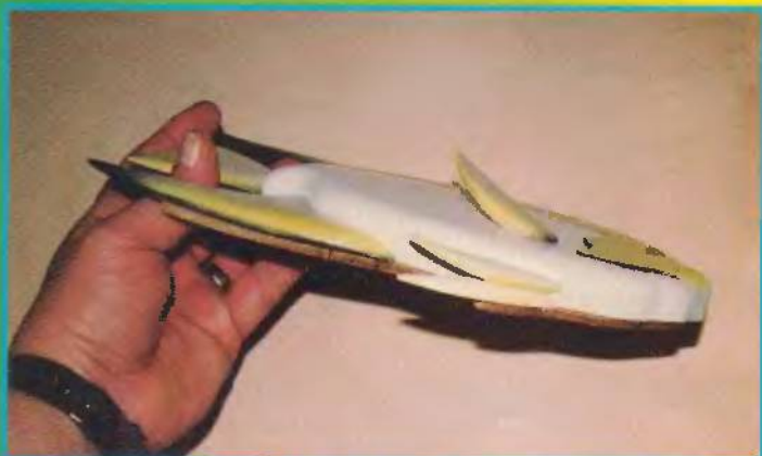
Fig. 10. Edge view showing the plywood back and the fin contours.
