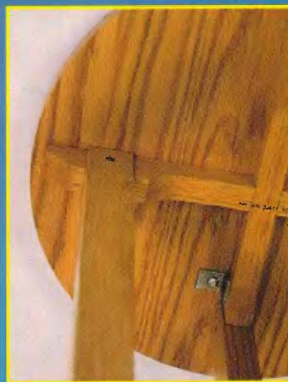
Bottom view of the table, showing the bridle and lap joints as well as one of the z-clips which secures the top
