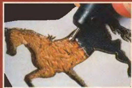
Fig. 2. Use a round burr to rough out the pattern.
