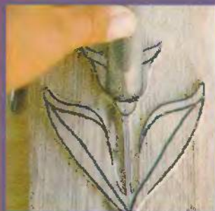
Fig. 2. Make the rounded stop cuts at the base of the petals and at the base of the calyx with the No. 7-25mm gouge.
