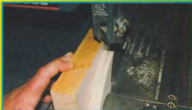
Fig. 3. When resawing the fins and tail, make sure the wood makes contact with the saw table.
