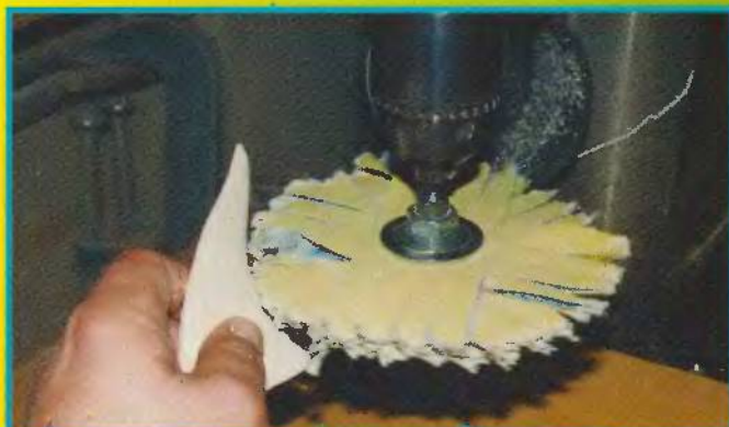
Fig. 5. A flutter wheel will make quick work of smoothing each piece.
