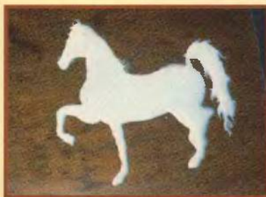
The finished pour should be about 1/16 " higher than the wood surface.
