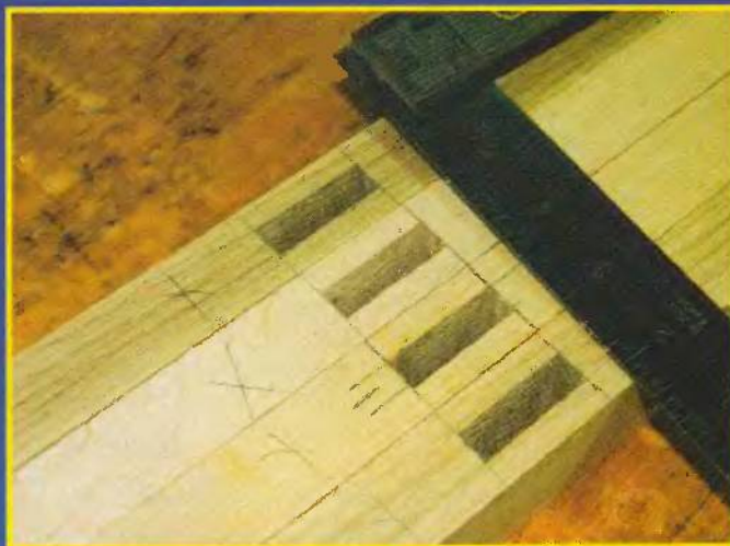
Fig. 1. Carefully mark the location for the mortises, then cut them as shown. The "X" denotes the inside edge of the leg.
