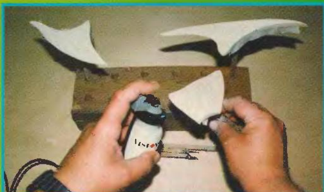
Fig. 6. Cover the edges to be glued with masking tape, then basecoat the pieces. Attaching an X-acto knife blade to a slotted wood piece for a handle will make spraying the pieces simple.
