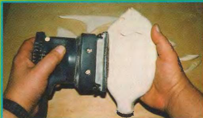
Fig. 4. Sanding will create a smooth finished project; oversanding will create gaps between the pieces.
