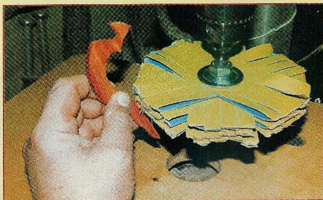
Fig. 2. Lightly sand both sides of the ornament, including the section where the wing meets the body, with a flutter wheel to ease the cut edges.
