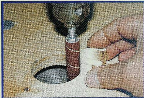
Position small sanding drums close to the edge of the auxiliary table.
