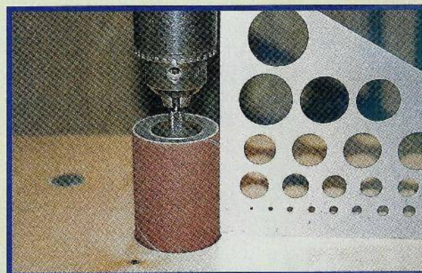
Make sure the sanding drum is perpendicular
