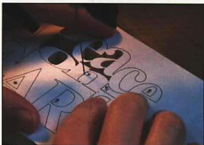
Step 6. Using the scroll saw and your blade of choice, carefully make all the interior cuts of the design. (Leaving the surrounding wood intact provides you with a uniform edge, which helps you pivot and maneuver the wood as you feed it into the blade.)
