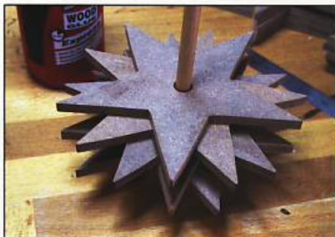
Step 10. Stack the five large stars on the dowel in a staggered fashion, pressing down lightly to glue them in place.
