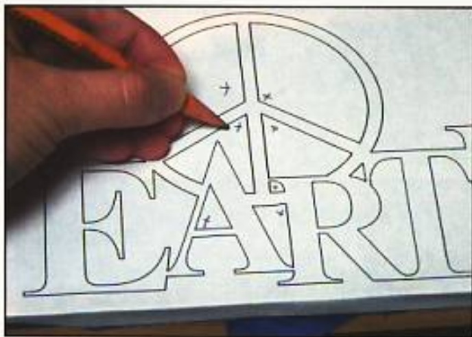
Step 3. Using a pencil, mark an "X" at each point where a blade entry hole will have to be drilled.
