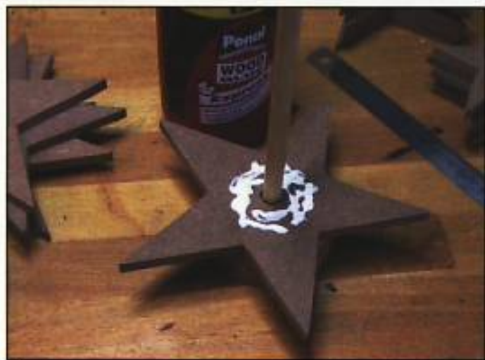
Step 9. Apply wood glue to the center area of the five largest stars.
