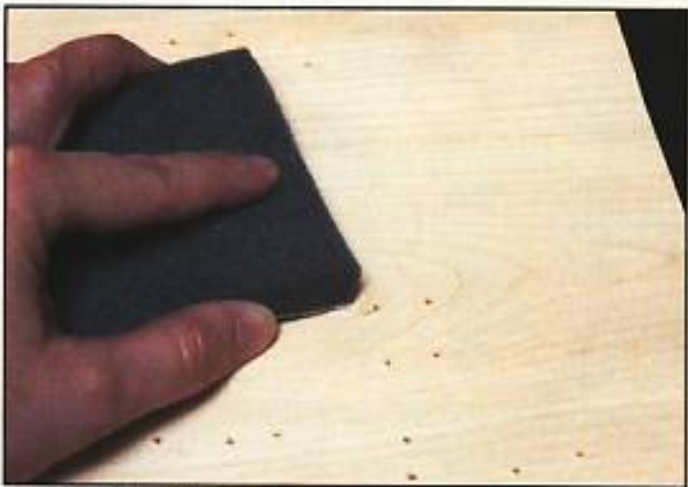
Step 5. After drilling, use a sanding block to remove any tear out from the back of the work piece. This will make feeding the blade through the holes much easier.
