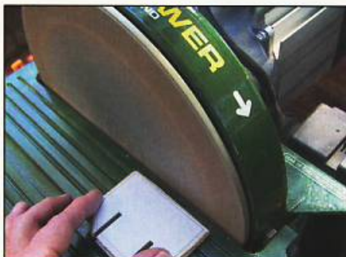
Step 10. Use the disc sander to sand the straight edges of the feet pieces up to the pattern lines.
