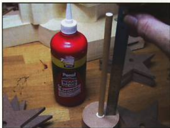
Step 7. Insert the piece of dowel into the hole in the base, and glue in place using wood glue. Let dry.
