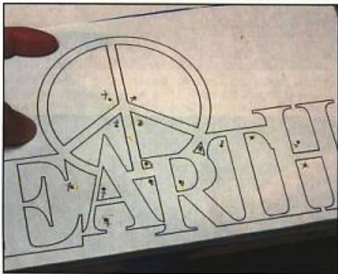
Step 4. Drill a hole at each marked point.
