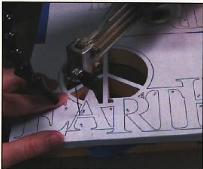
Step 3. Using a pencil, mark an "X" at each point where a blade entry hole will have to be drilled.
