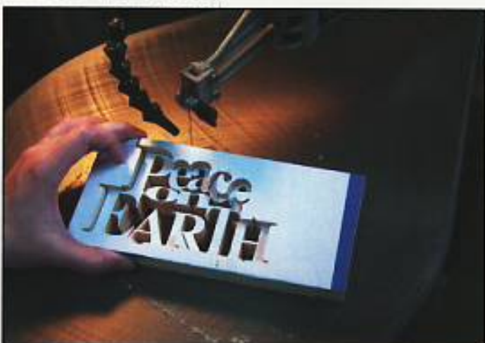
Step 7. After completing the interior cuts, carefully cut along the perimeter of the design, releasing the word art from the surrounding wood.
