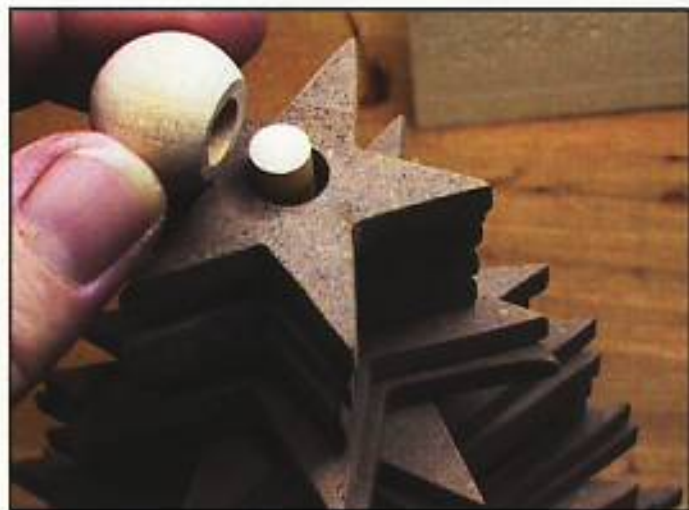
Step 8. Dry-fit the star pieces onto the dowel, and adjust the length of the dowel as needed.
