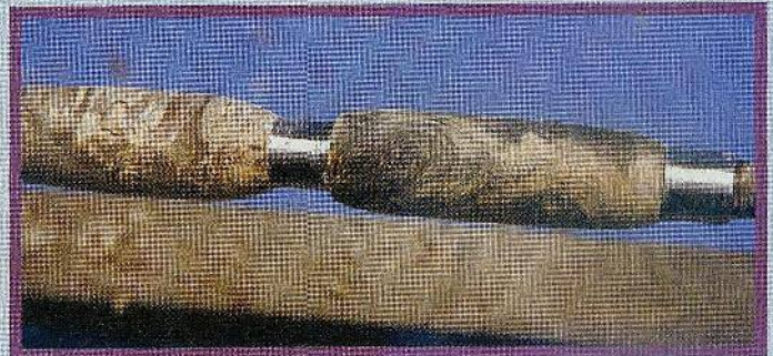
Fig. 4. Once your patch dries, scrape the excess from the blank with the exacto knife. Turn the lathe on low speed and sand, starting with coarse sandpaper. Finish normally, slowly increasing the lathe speed as you progress through the grits, checking frequently for the condition of the flaw and the transition from blank to bushing. This method is particularly successful with Staburized (tm) blanks. Standard turning wood blanks may respond differently, so keep a notebook nearby to keep track of your results. Happy turning!
