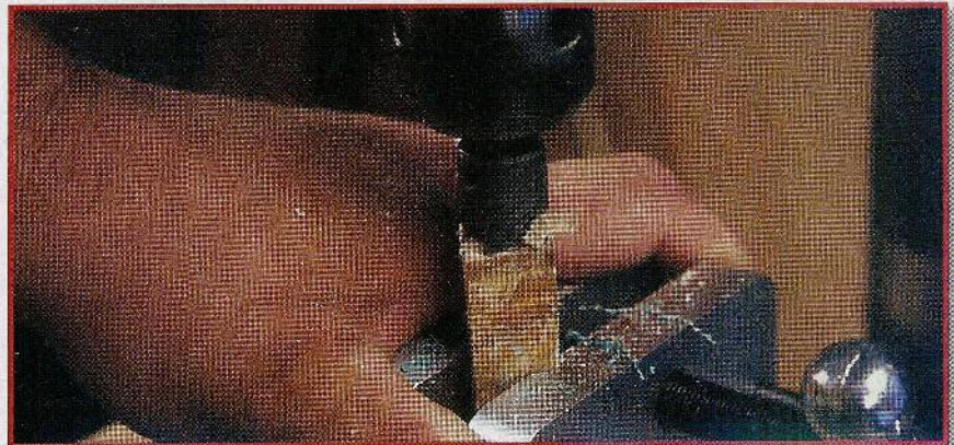
Fig. 3. Use the barrel trimmer with the 10mm pilot shaft to true and trim both ends.
