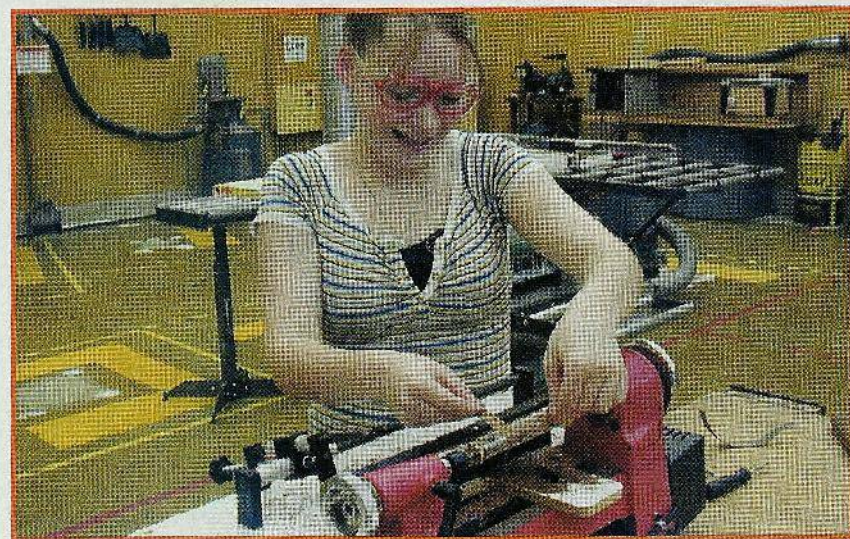
A student sands her project after turning the barrels. The sanding process uses graduated sandpaper grits, a typical step in wood finishing.
