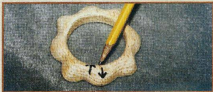
Fig. 4. Shape a gentle radius on the inside and outside edges of the branches.
