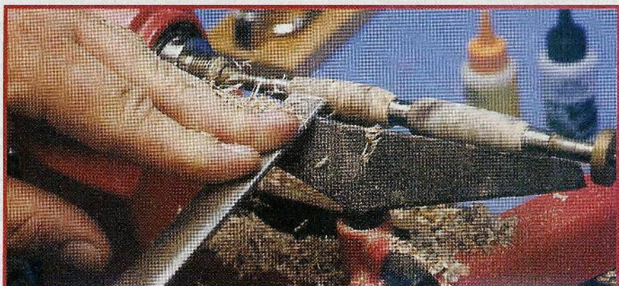
Fig. 6. Continue shaping the key rings using a skew chisel until you are satisfied with the smoothness and shape.
