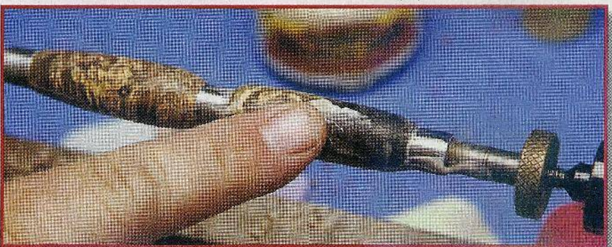
Fig. 8. Apply Shellawax Cream while the pen is on the lathe.
