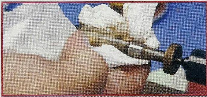
Fig. 9. Begin buffing with the lathe on medium speed, and move quickly to high speed for a nice shine.
