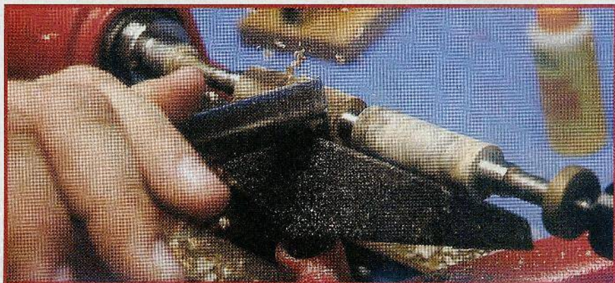
Fig. 5. Use your rough out gouge to round out the blanks.
