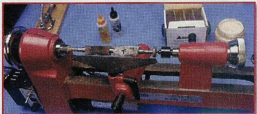
Fig. 4. Load the mandrel with two key ring blanks.
