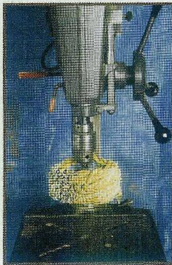
Fig. 4. A drill press fitted with a flapper wheel disc for sanding pieces that have already been contoured.
