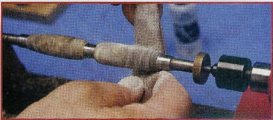
Fig. 7. Turn the lathe speed down slightly and begin sanding with cloth-backed sandpaper.
