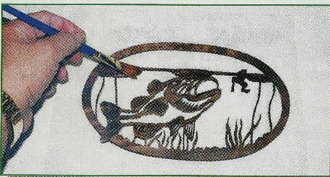
Fig. 7. Use a small brush to apply Watco Danish oil to the pieces.
