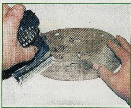
Fig. 6. Periodically sand the "fuzzies" off the back of the workpiece as you are sawing.
