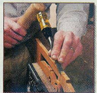
Fig. 4. Use the chisel to remove stock to the desired depth.
