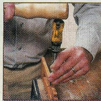
Fig. 3. Start making the mortises by making plunge cuts with a small chisel.
