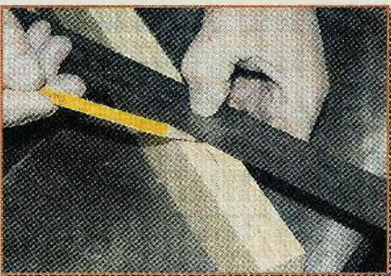
Fig. 9. Draw a centerline down the middle of each cross slat. The easiest and most accurate method is to place a rule on the stock so that the graduation lines for two whole numbers (I used the 4" and 6" graduation marks) are aligned along the opposing edges of the stock. The centerline in my case was located on the midpoint, or the 5" graduation mark.
