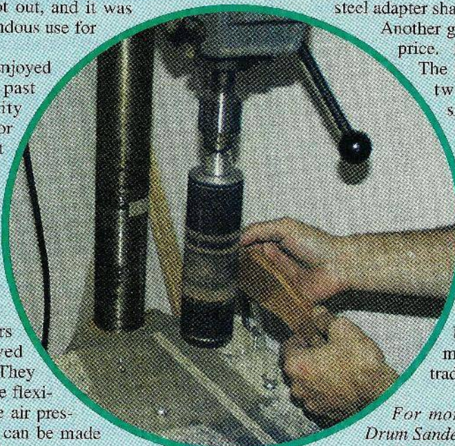
The Flex Drum Sander can be easily mounted in a drill press
