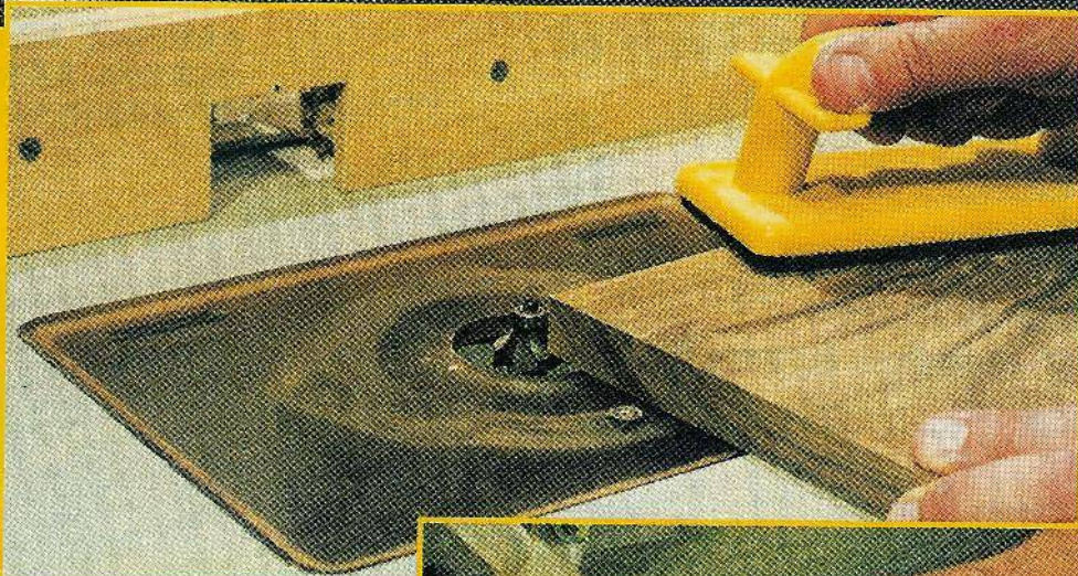
Fig. 1. Using a 1/4" roundover bit to shape the front edges of the plaque.
