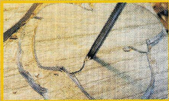
Fig. 5. Making an oval cut with the No. 9-4mm gouge to carve out the "eyes" of the grape leaf.
