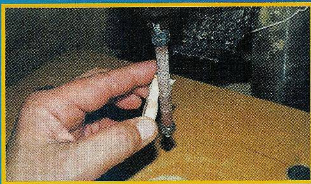
Fig. 8. A 1/4"-Dia. x 4"-long sanding arbor is useful for contouring the parts of the hammer as shown in the contour drawings located in Full Size Pattern Section No. 2.
